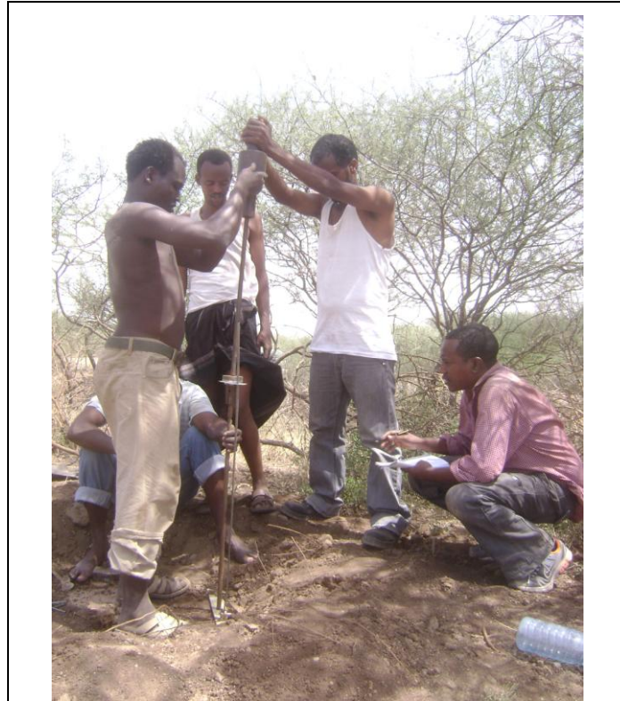
Picture 3.3 Conducting DCP on site (at Sta. 41+000)
