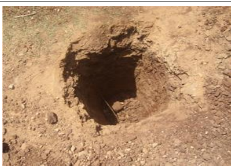
Picture 3.1 Test Pit Investigation (at Km 45+000, C/L)
