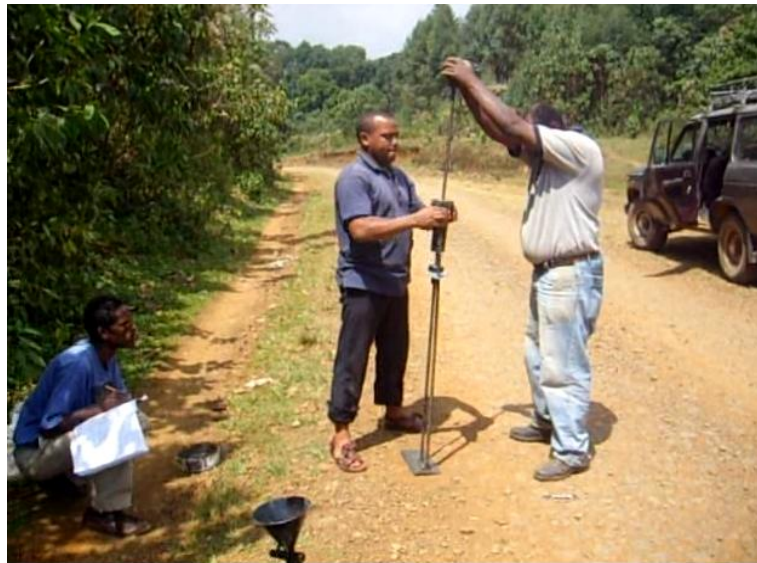
Picture 2.1 Application of DCP in Pavement Investigation (Gravel Road)
