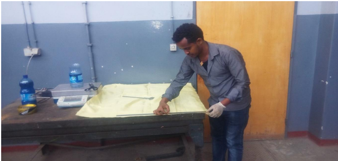
Figure 3.4. Kevlar and E-glass cut with dimension is 229\text{mm} \times 229\text{mm} \times 20\text{mm}
