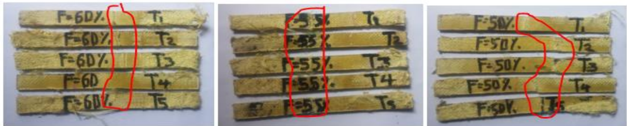
Figure 3.21. After tensile test pieces' different composition ratio of fiber/epoxy for tensile test
