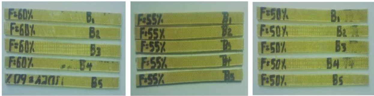
Figure 3.18 Taste pieces' different composition ratio of fiber/epoxy for flexural taste
