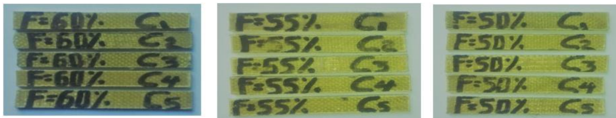
Figure3.16 Taste pieces' different composition ratio of fiber/epoxy for compression taste
