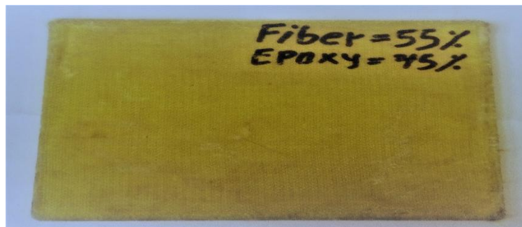
Figure3.8. Hybrid composite plate of fiber 55% and matrix 45%.
