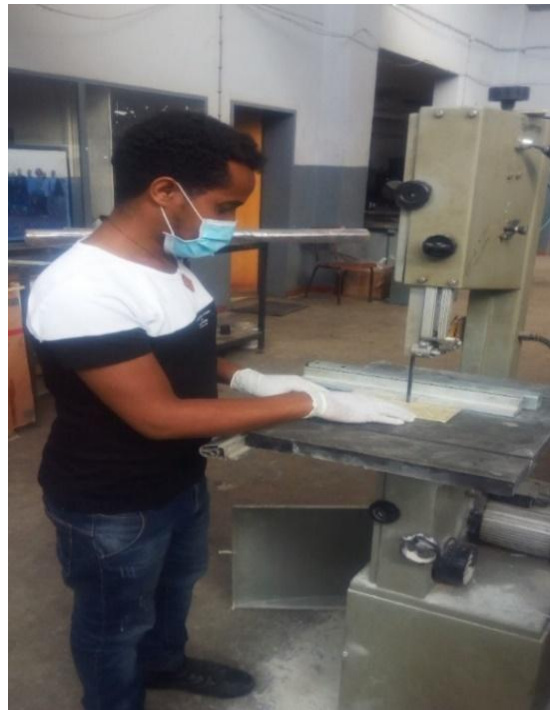
Figure 3.12. cutting taste pieces using band saw machine.
