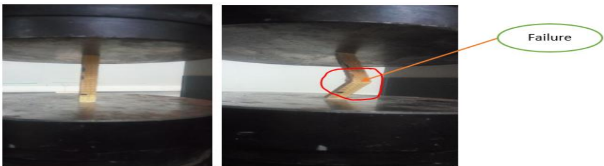
Figure 3.40. Compressive strength taste set up
