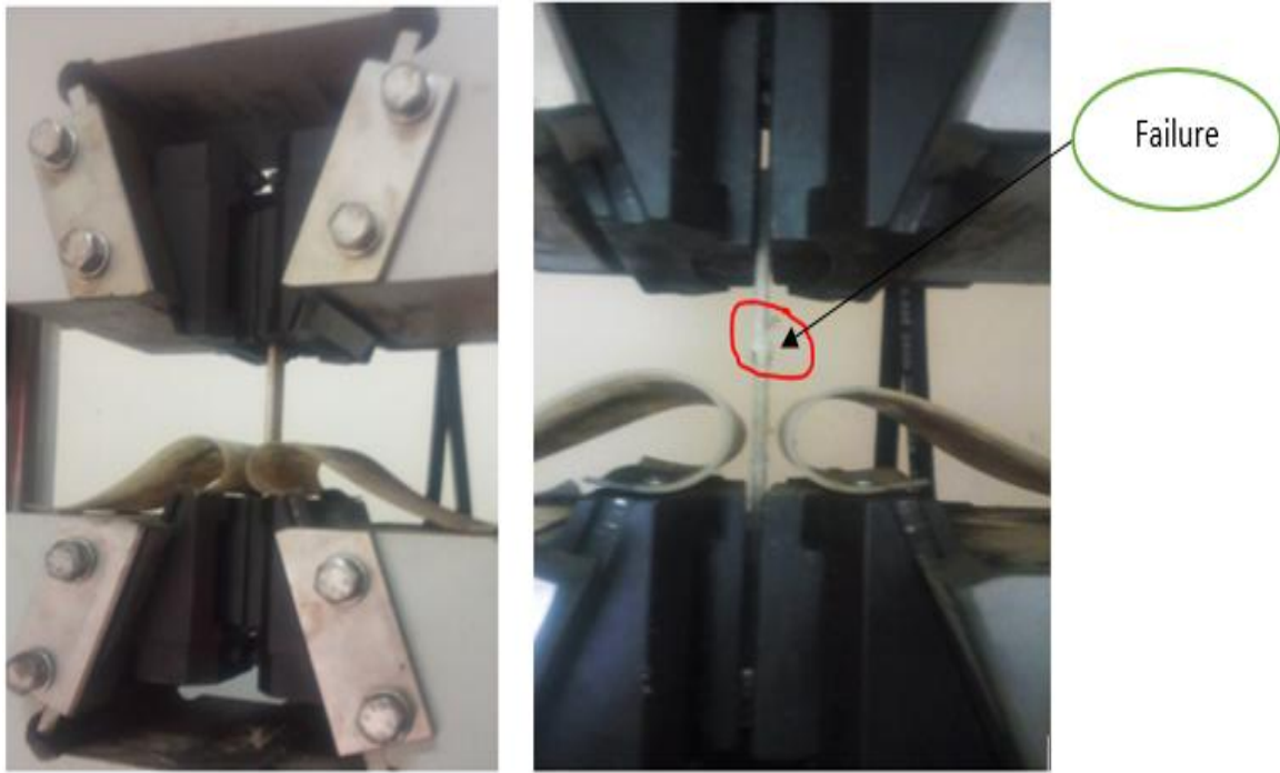
Figure3.20. Tensile strength taste set up
