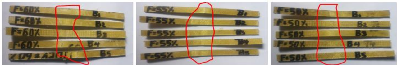
Figure 3.31. After flexural/bending taste that show pieces of failure for different composition ratio of fiber/epoxy
