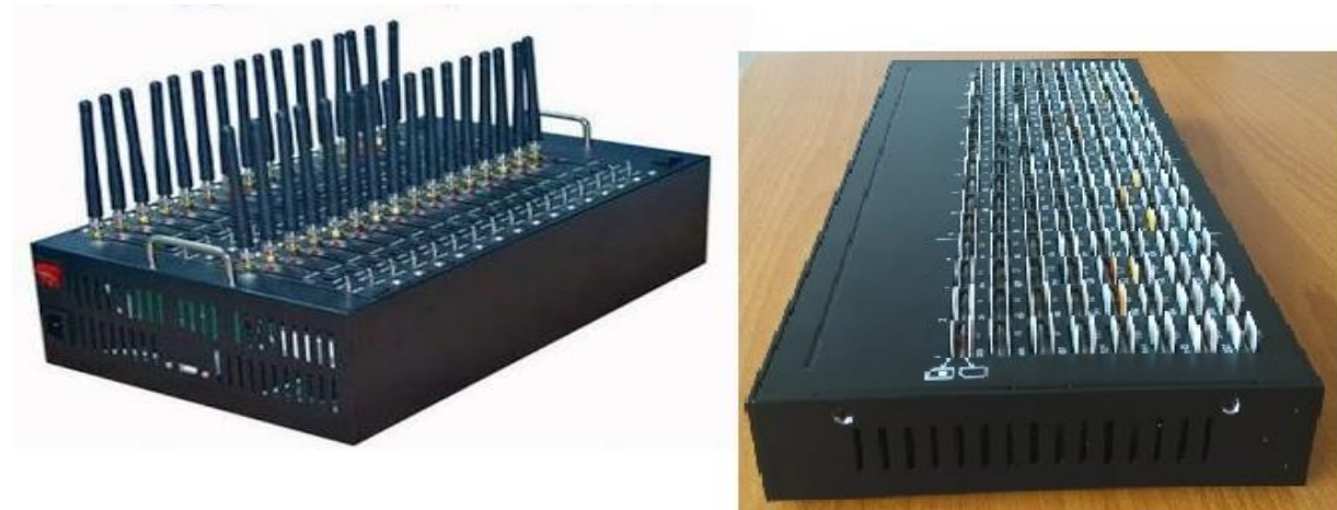
Figure 1: Two models of SIM box device (New module 32 SIM card gsm SIM box and 128 SIMs cards call center SIM box device)
