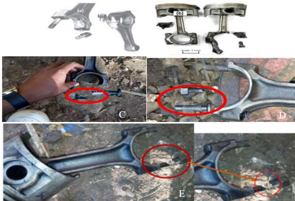
Figure 1.1: Connecting rod bolts failure (a & b) [3] [4] and observations from Henok Garage Center (C, D and E) image by Bikila
