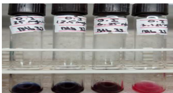
Figure 10 – The color change of resazurin in the presence of O. integrifolia extract against btb33 strain
