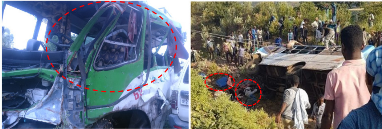
Figure 1.1: Damaged midi-buses structure, fatalities, and injuries during rollover accidents (Source: Ethiopian Insurance Corporation in 2017(left) and field photo, Geregera town in 2019(right))
