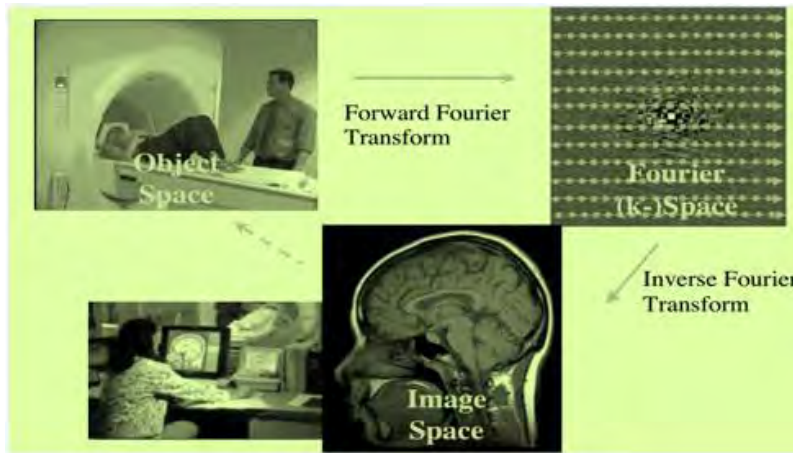
Figure 4.2: The MR imaging process can be viewed as forward and inverse Fourier transforms [Curtsy of Medical Image Processing Overview Hongmei Zhu, University of Calgary PP.2]
