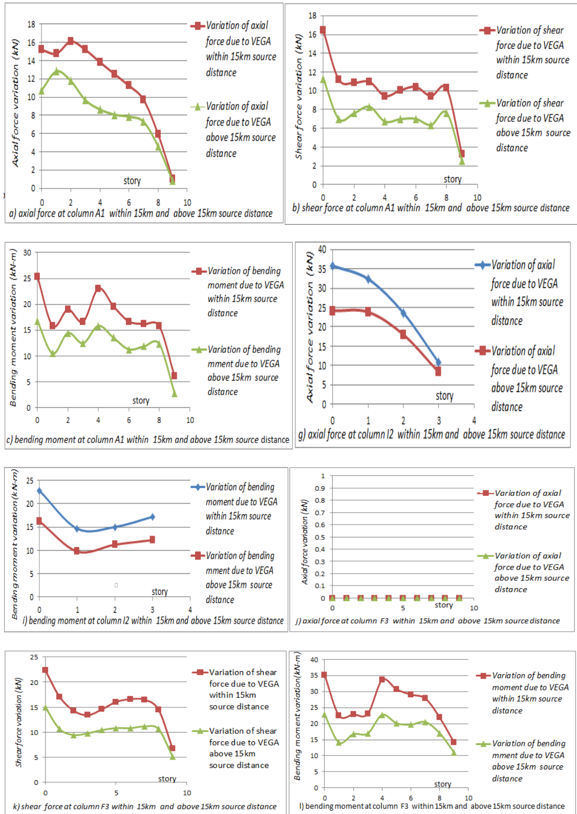
Figure A: Effect of VEGA on building response due to difference source distance
