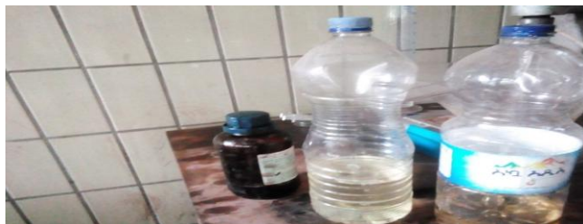
Figure 20 Shows reagents used in the flotation experiment n-octanol ( \text{CH}_3(\text{CH}_2)_7\text{OH} ), kerosene and sodium silicate ( \text{Na}_2\text{SiO}_3 ) respectively.
