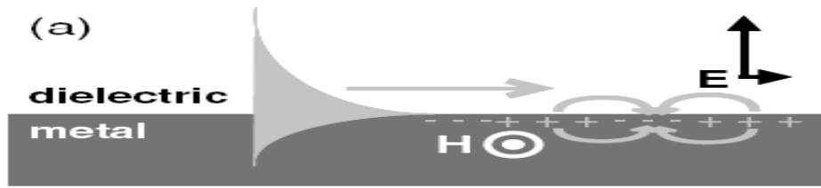
Figure 2.7: Schematic representation of a SPP propagating along a metal-dielectric interface and orientations of electric and magnetic field components).
