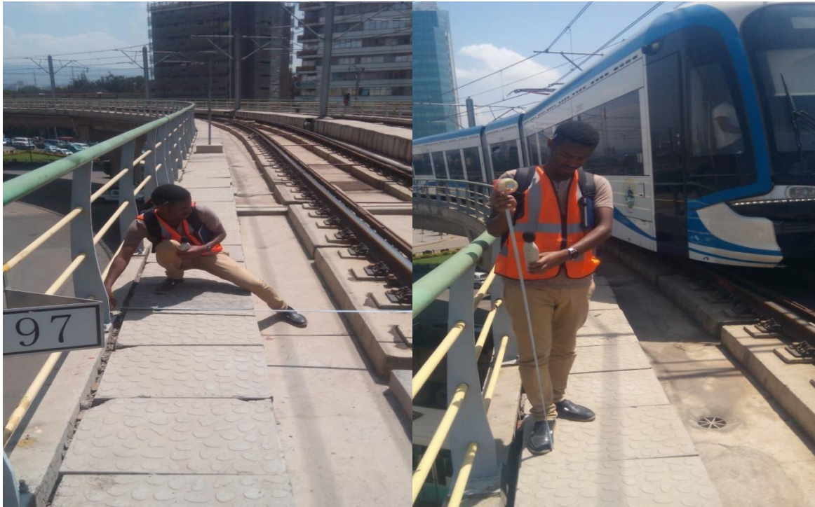
Figure 12: Site measurement using sound level meter.
