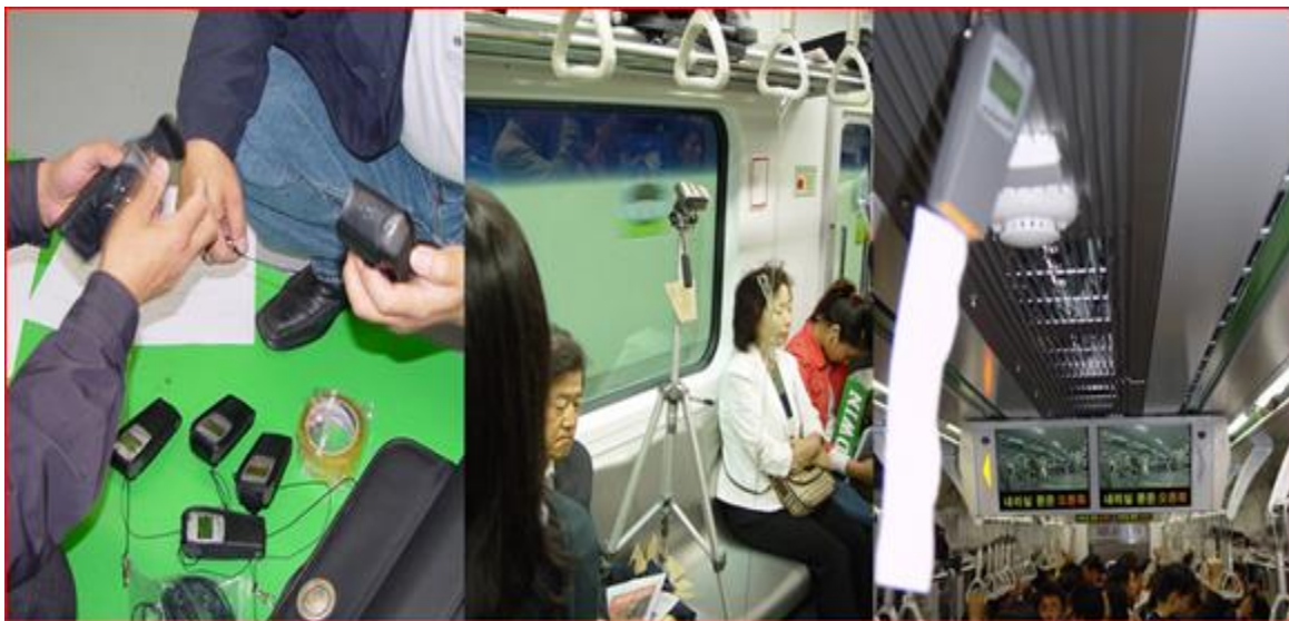
Fig 2.3: Measurement of co 2 concentration at indoor air
