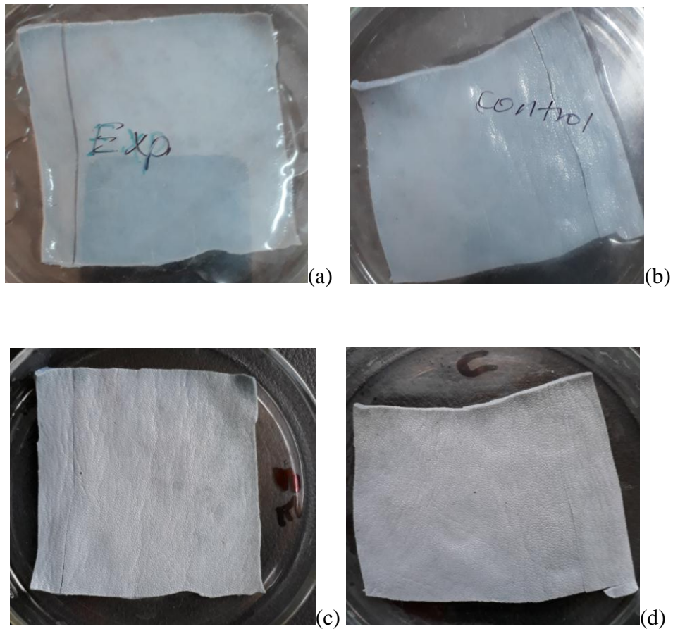
Figure 26: Leather cuts in the humidity chamber; 0 day of experiment (a) and control (b) and 15 days of experiment (c) and control (d)
