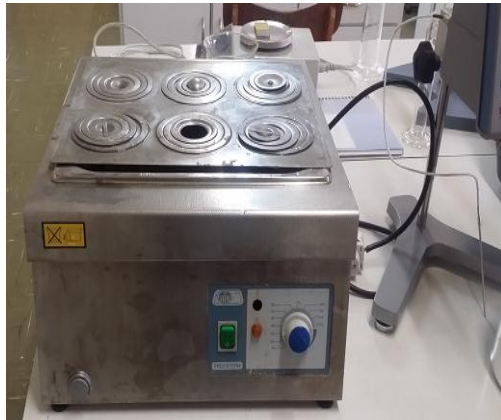
Figure 3.4.3.3a: Water bath used for temperature control
