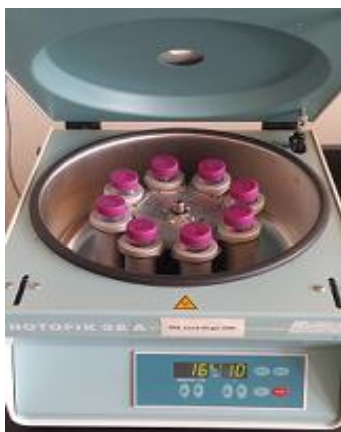
Figure 3.4.1.2 Centrifuge used in the WHC determination
