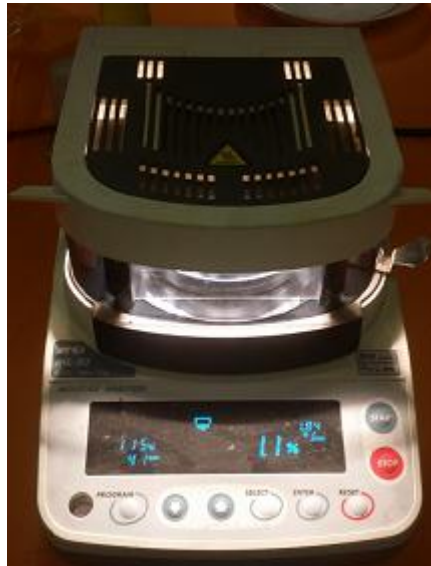
Figure 3.4.3.7: Instant moisture analyzer
