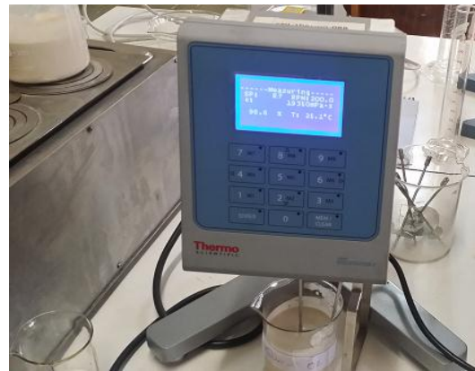
Figure 3.4.3.3b: HAAKE Viscometer used for Viscosity measuring
