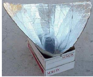
Figure 1-1: a) box type solar cooker, b) panel solar cooker, c) parabolic solar cooker, d) funnel solar cooker, e) Scheffler Cooker [9]
