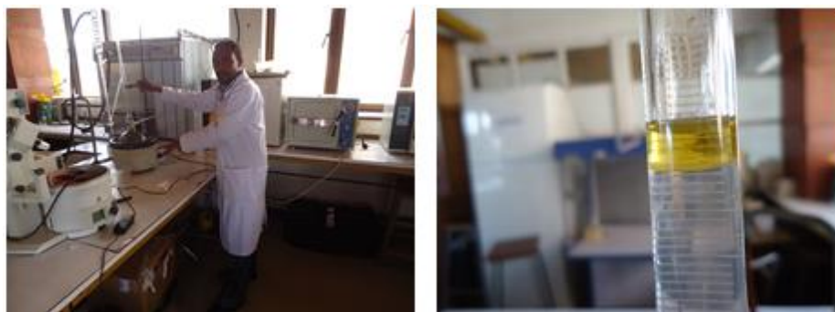
Figure 17: Water distillation of Thymus powder (dry weight) using clevenger type apparatus
