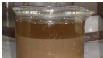
Figure 3.3 Adsorption of Clay treated lubricant
