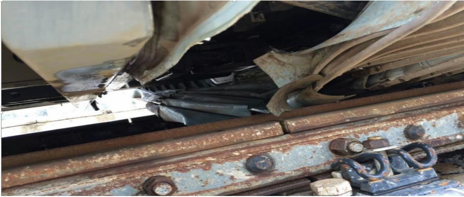
Figure 2. Gangway system folding bellows lower down to the rail.
