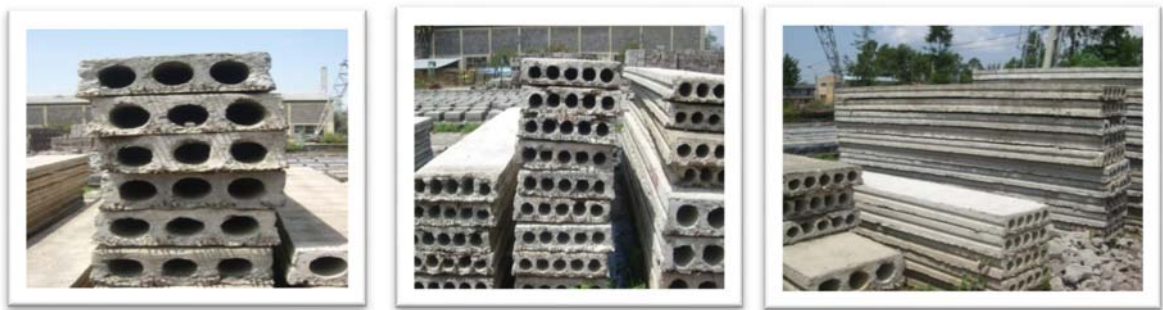
Figure 2.13 Typical prestressed hollow core concrete floor units produced in KCMPE Addis Ababa
