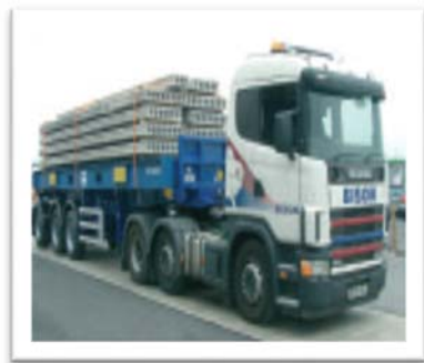
a) Transporting of hollow core slab
