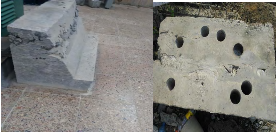
Figure: 4.11 the dam prototype and the core point on the dam surface.
