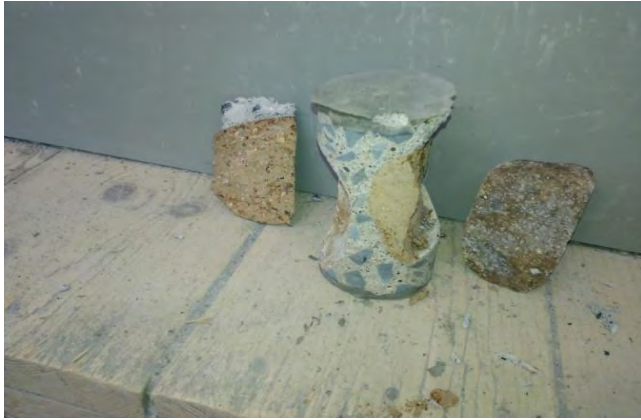
Figure: 4.13 Compressive strength failure mode of the core sample.
