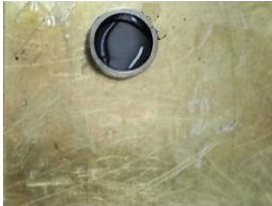
Figure 6: Preparing Asphalt Specimens for the DSR testing
