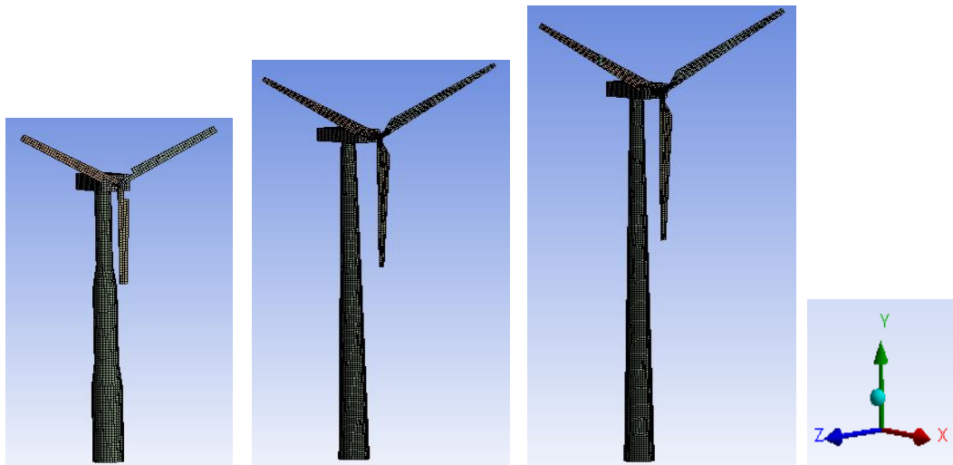
Figure 4.2: Mesh of 65kW, 1.5MW and 5MW wind turbines from left to right respectively.
