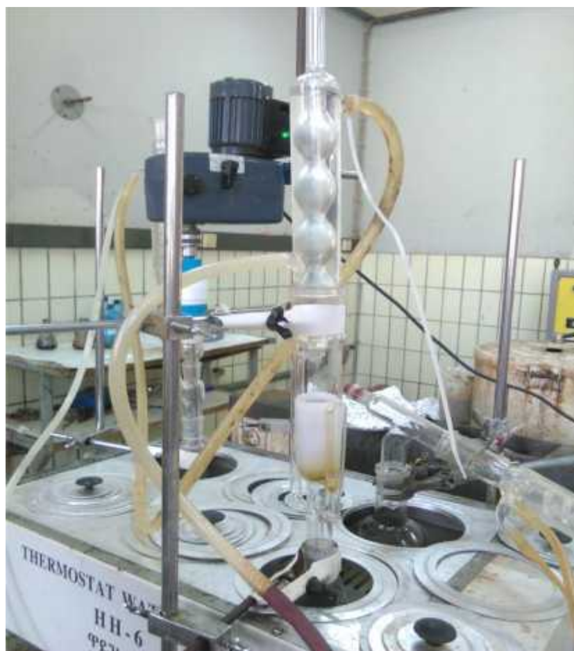
Figure 3-1: Experimental setup on Soxhlet extractor
