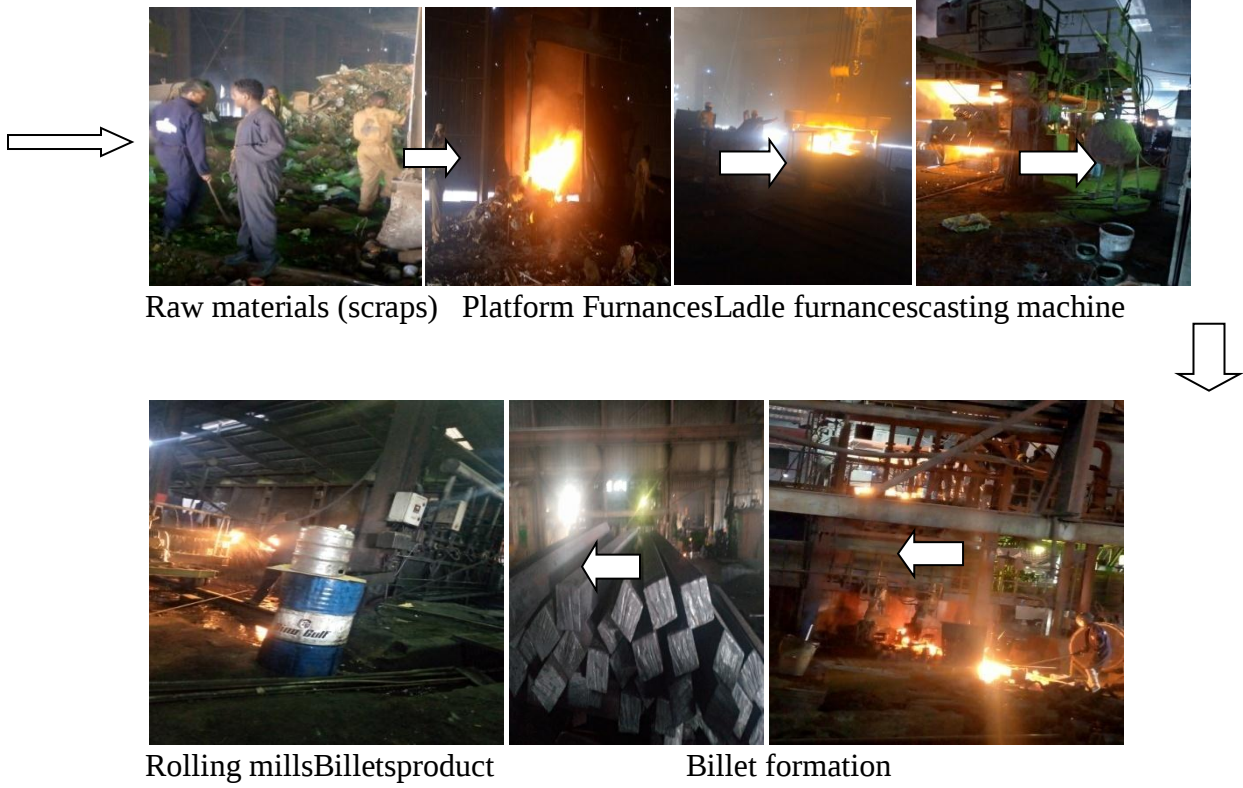
Figure 9: Work processes of Habesha Steel mill
