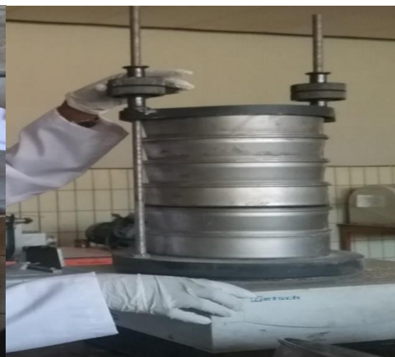
Raw material preparation (Size reduction and sieve analysis of cotton and coffee husk)
