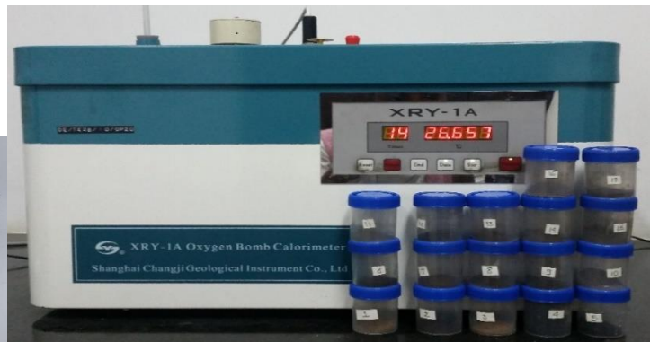
Bomb calorimeter for determining calorific value
