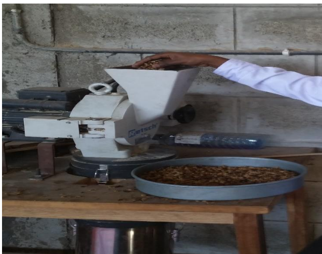
Raw material preparation (Size reduction and sieve analysis of cotton and coffee husk)
