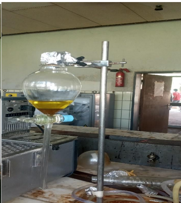
Separation of Biodiesel and glycerol
