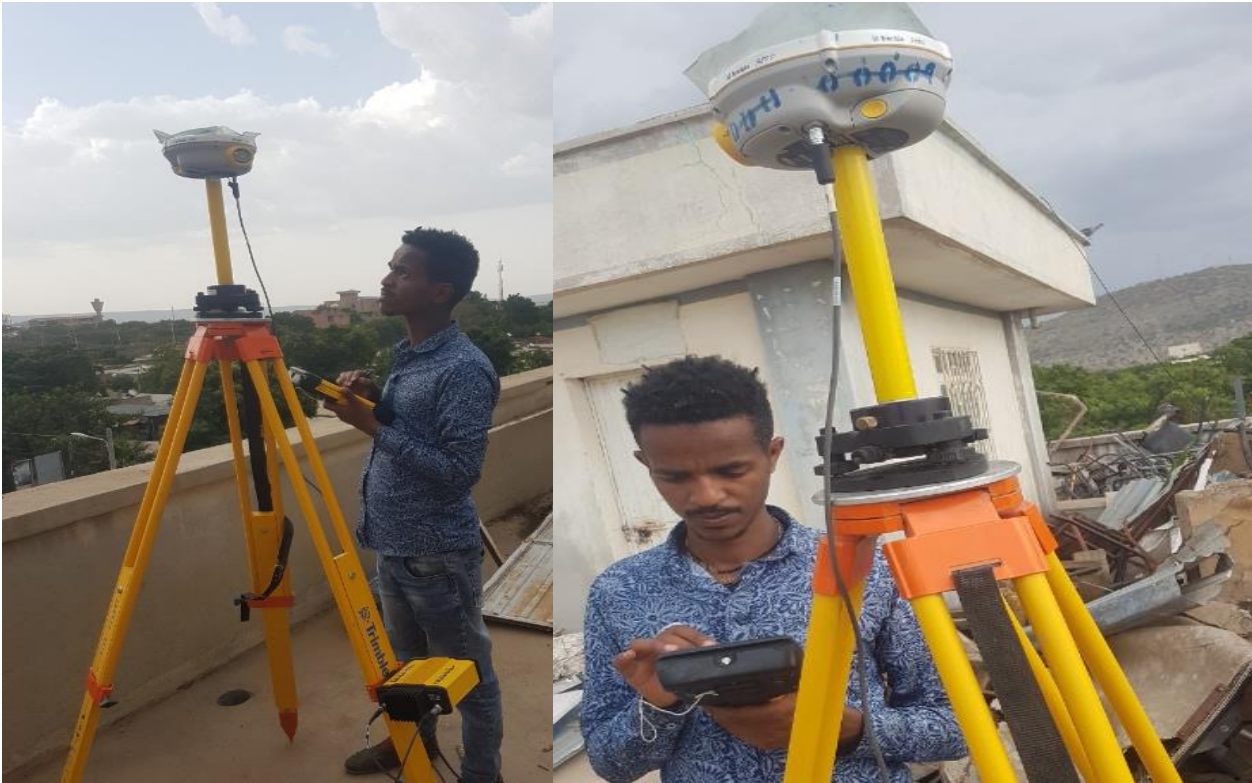
Figure 3.2 Connecting radio link with base and rover receiver
