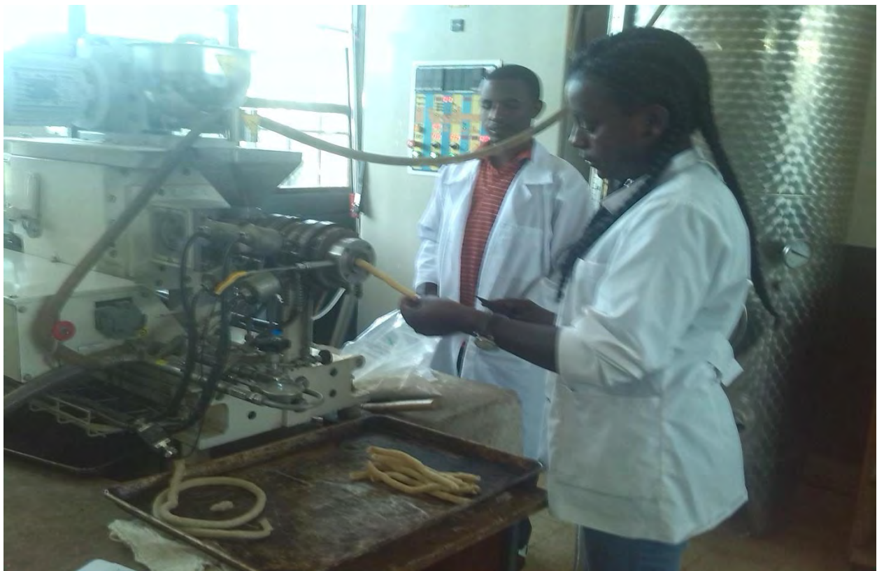
Fig.2. Extruding process and collecting the extrudate
