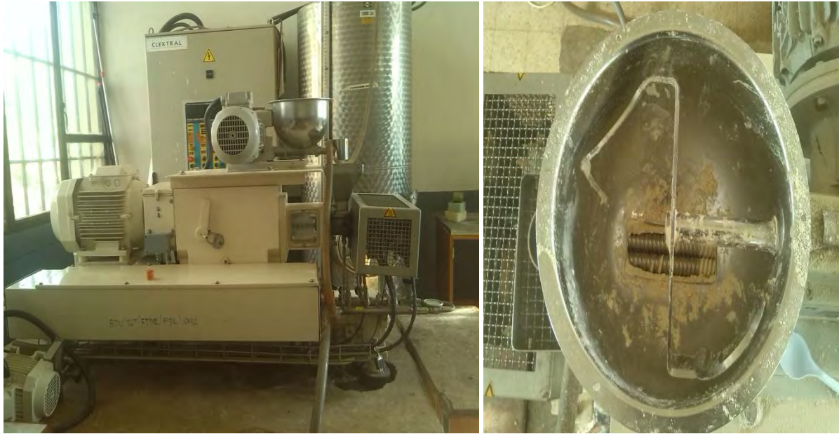
Fig.1 Extruder Machine and extrusion feeder with twin screw
