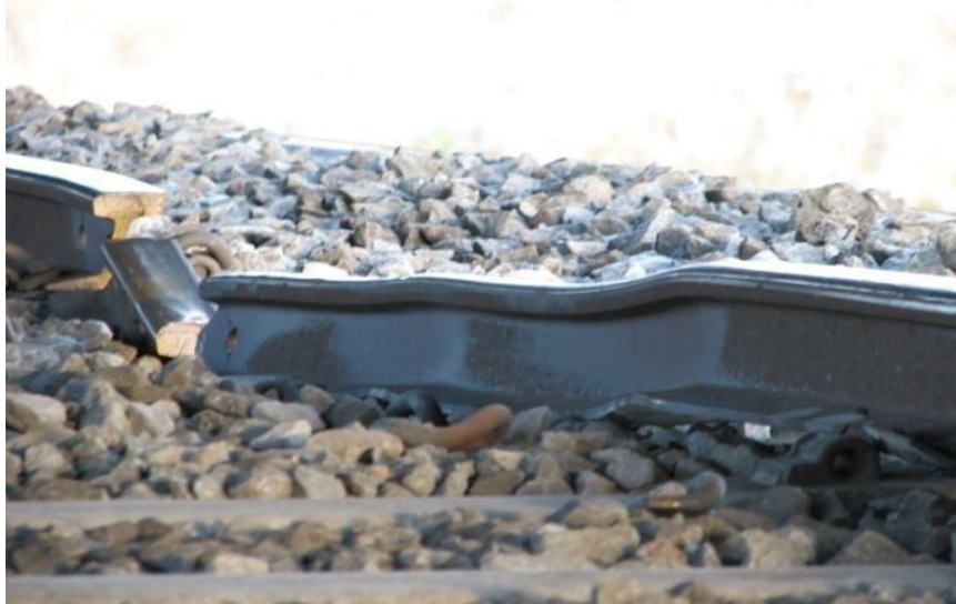
Figure 2.22: The fractured rail in-situ [Zhao et al, 2006]
