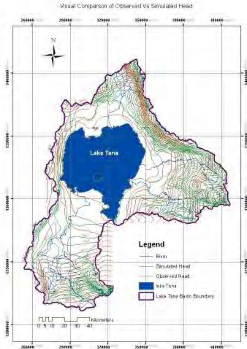
Fig: 6.2. Map of Observed Vs Simulated Hydraulic head of Lake Tana Basin
