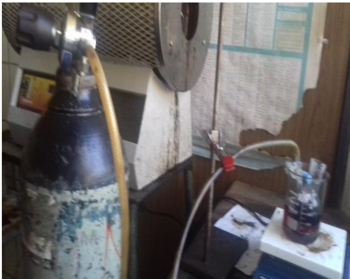
Figure B3: Experimental set up for Sulfonation of rice husk char
