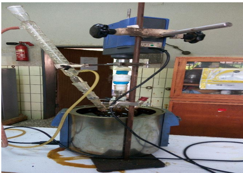
Figure B8: Experimental set up for esterification reaction
