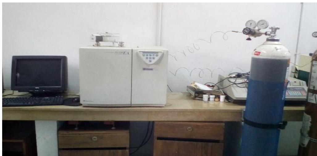
Figure B5: EA 1112 Flash CHNS/O- analyzer
