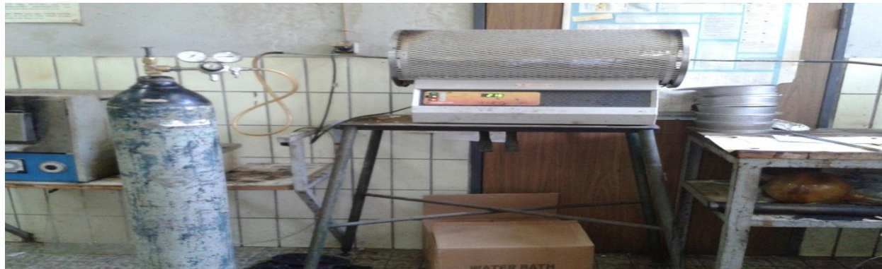
Figure B2: Experimental set up of the carbonization of rice husk
