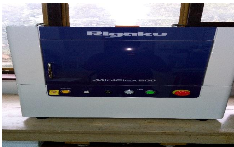
Figure B4: Rigaku, mini flex 600 X-ray Diffractometer
