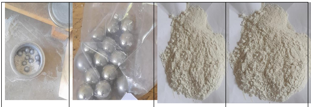
Fig. 5 The ball, ball mill and milled products of the sample
