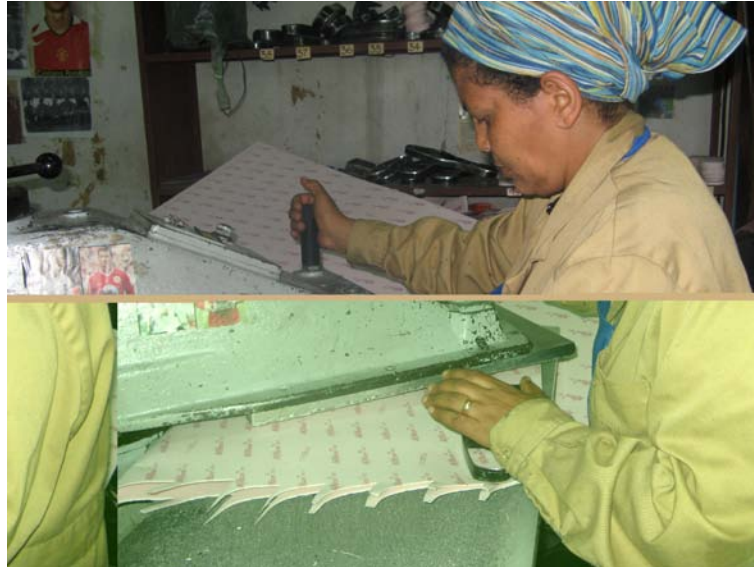
Picture2.5 Insole cutting operation
