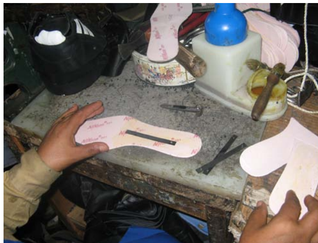
Picture 2.6 Attaching Shank to the insole
