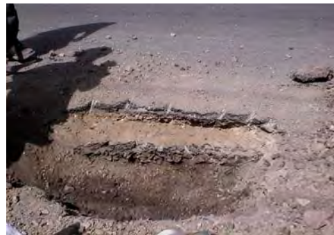
Figure 3.5 Test pit excavation on Test Road No 1
