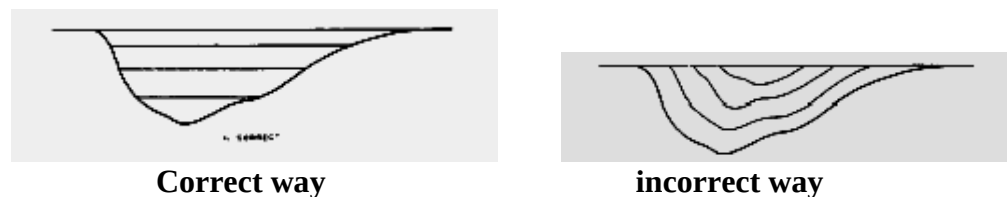
Figure 5.1 Back fill in deep depression
