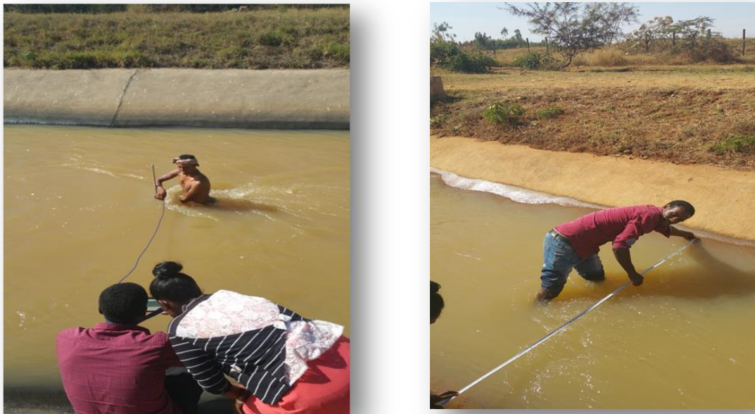
Figure 3 Discharge measurement of the main canal by using current meter (photo in 07/07/2010)
