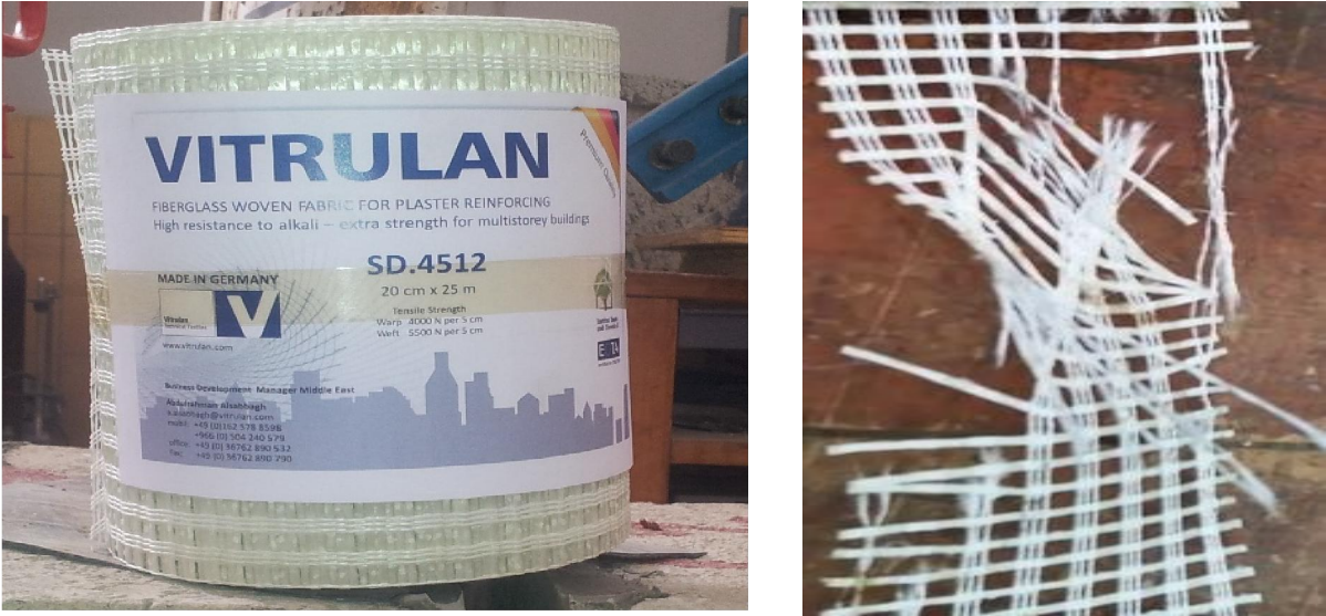
Figure 21 Roll of GFRP laminate and failure of FRP laminate
