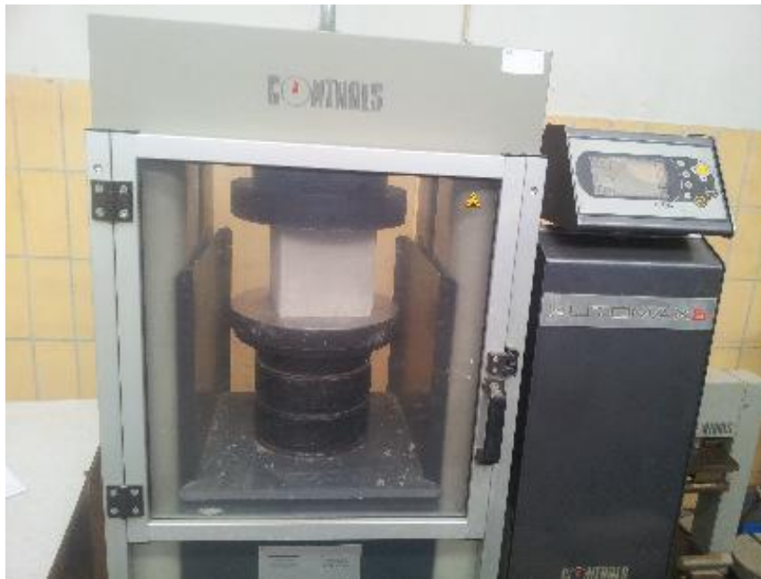
Figure 23 MCC computerized control console for testing concrete tensile strength
