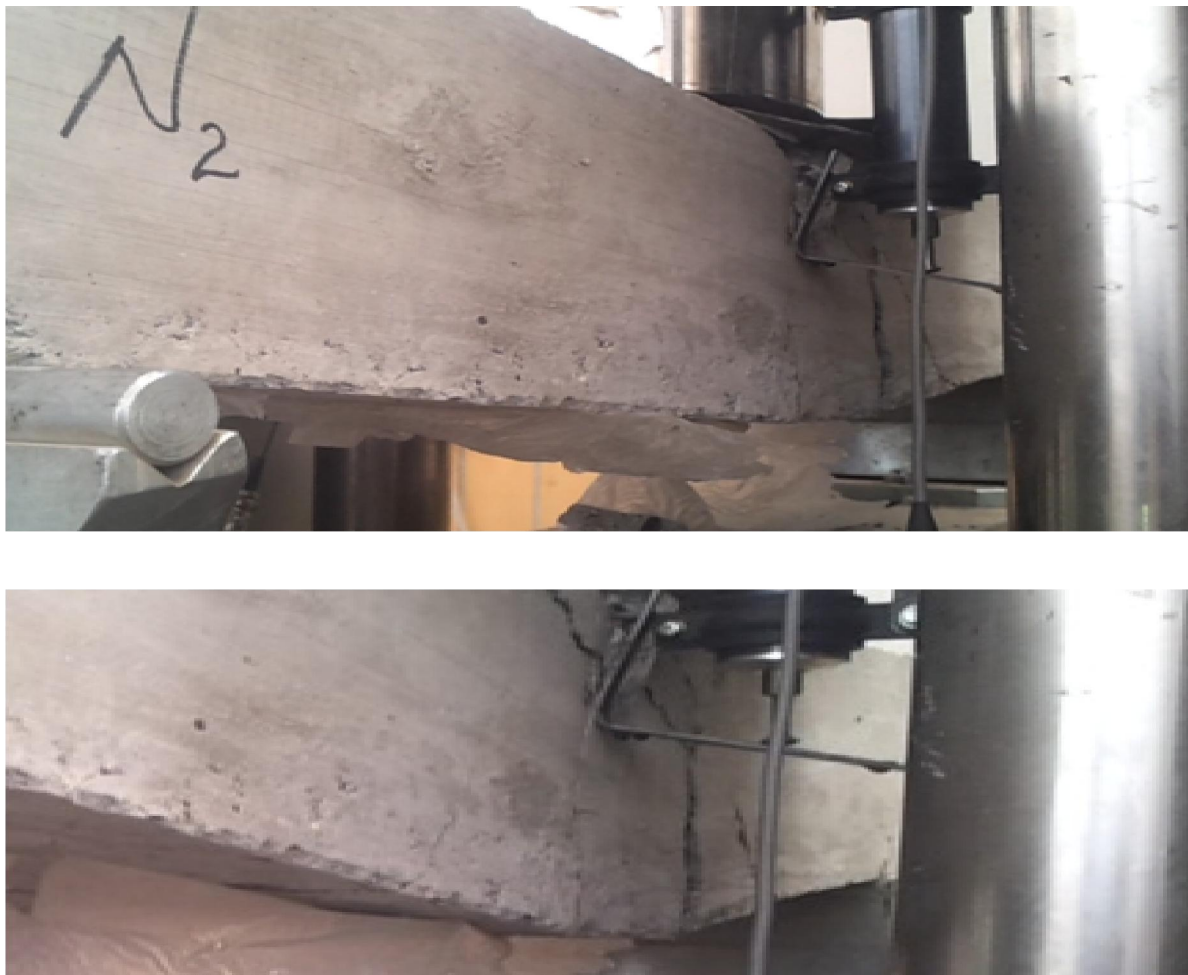
Figure 29 Flexural failures for control beam
