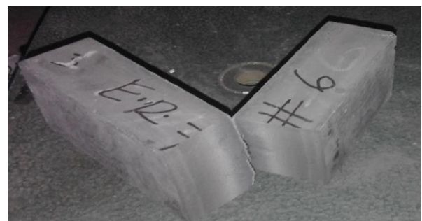
Typical specimen after tensile failure
