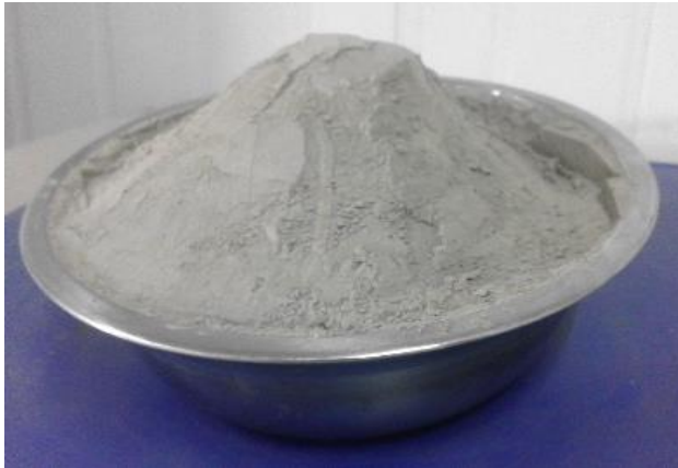
Ordinary Portland cement
