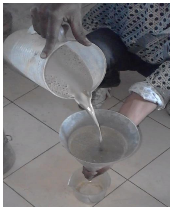
Figure 11: Cementitious grout being poured into Marsh cone funnel
