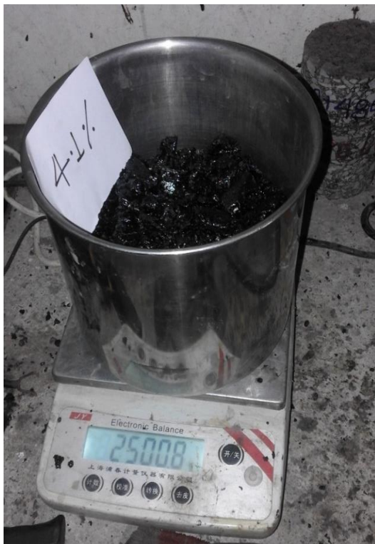
Weight measurement for Gmm
