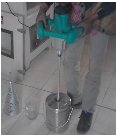
All ingredients added and being mixed
