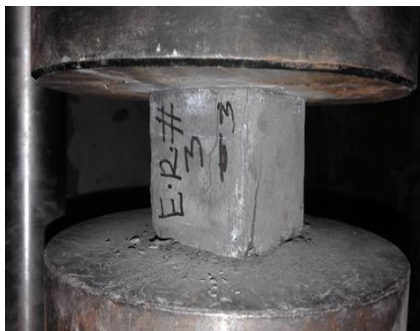
Typical cube under compressive
