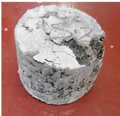
Typical grouted specimen after Marshal stability-flow test
