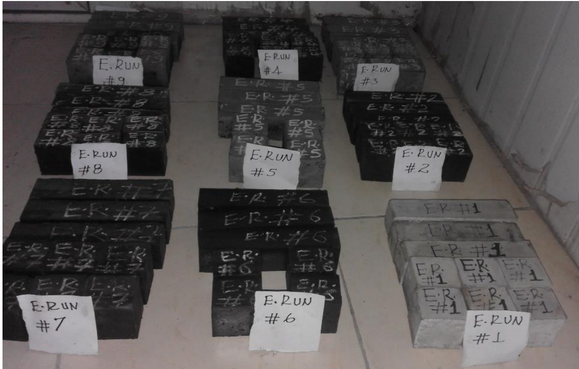
Grout mortar cubes and beams that are casted and being air cured.
