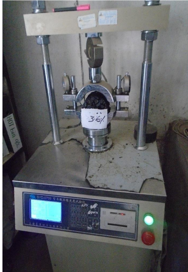
Typical porous specimen under Marshal stability-flow test
