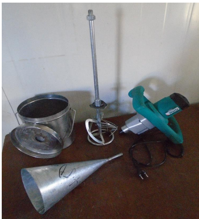
Figure 9: Photos of mixing bowl & its cover lid, mixing paddle, electric driven mixer and Marsh cone funnel
