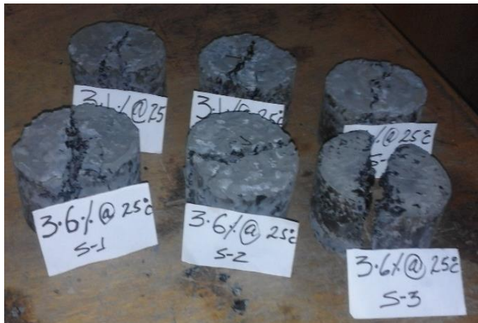
Grouted macadam specimens after ITS test
