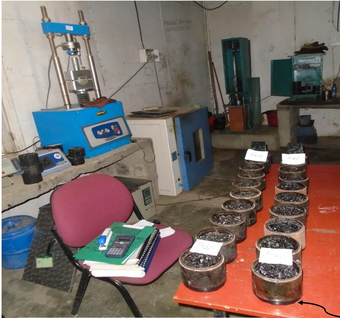
Compacted porous specimens ready for grouting
