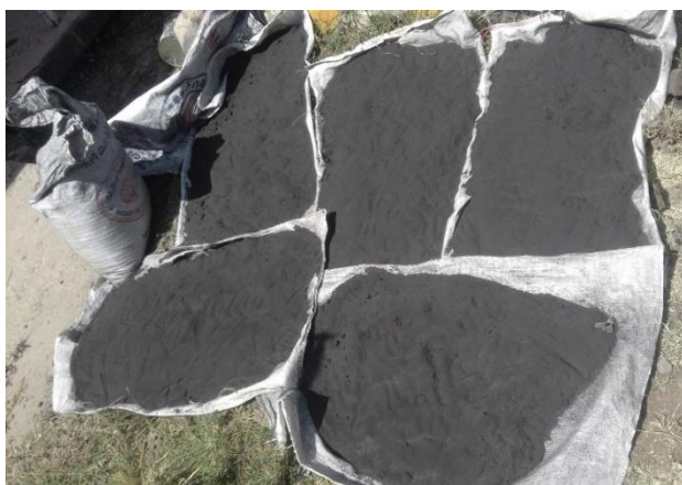
(a) Bagasse ash samples being air-dried
