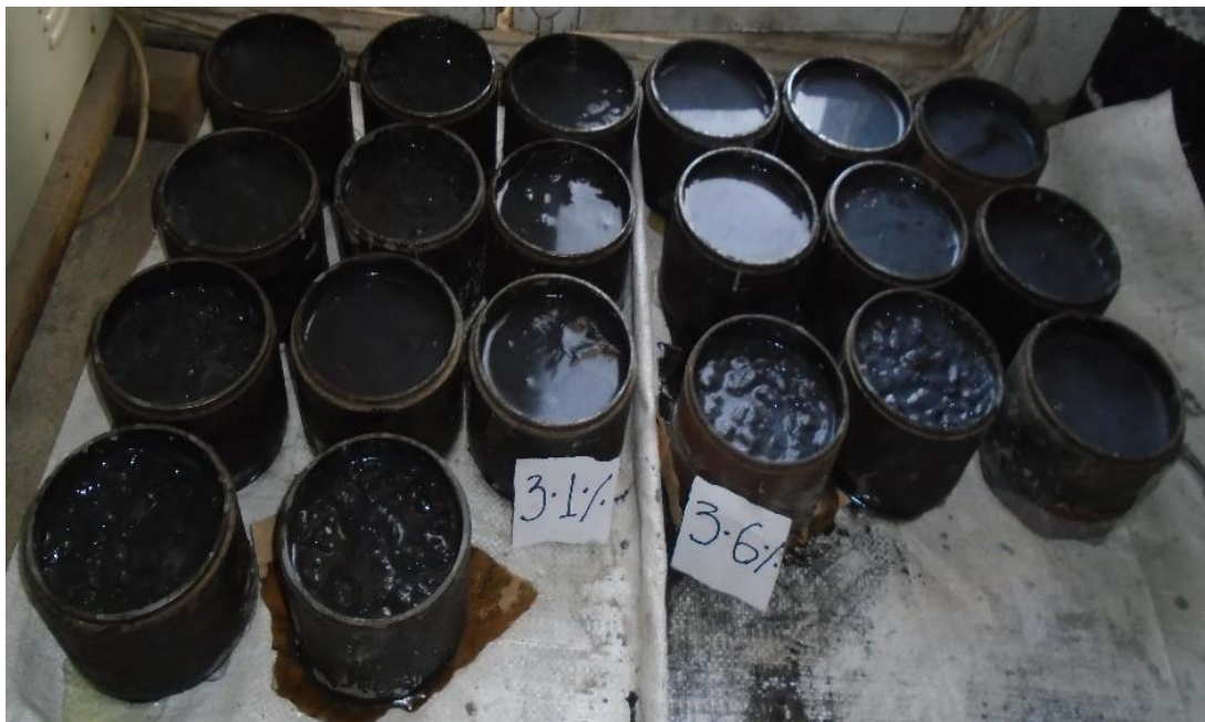
Grouted porous specimens immediately after two hours grouting
