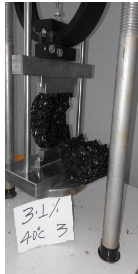
Typical porous specimen immediately after ITS test
