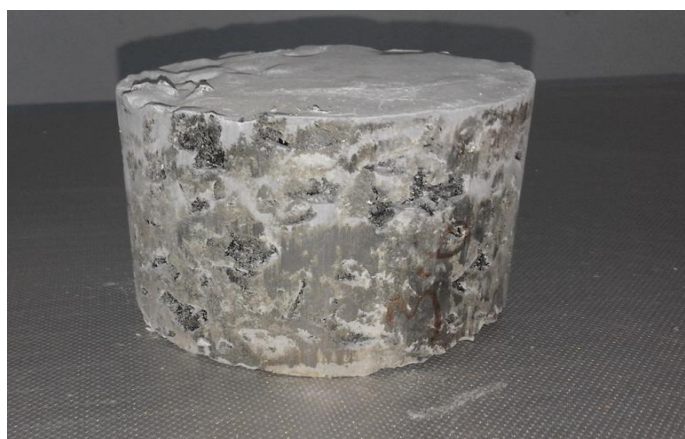
Figure 14: Typical grouted macadam specimen immediately after extrusion
