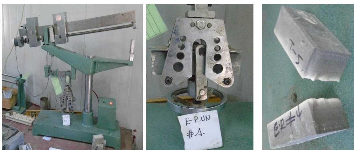
(a) Loading arm is raised to 1:10 (b) beam is inserted (c) beam after failure
