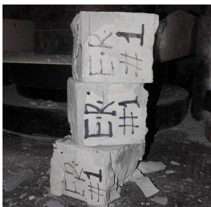
Cubes after compressive failure
