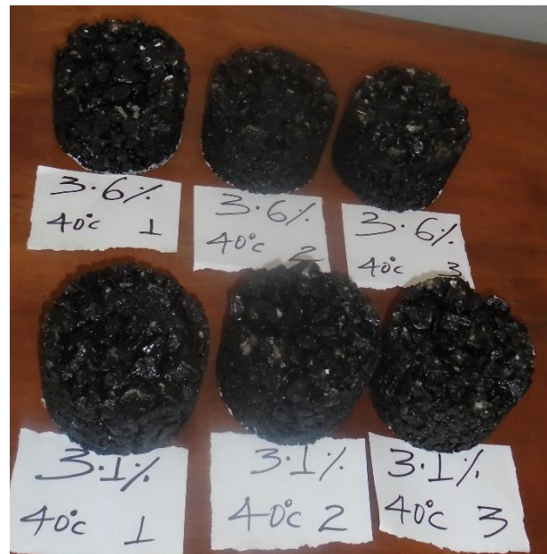
Typical porous asphalt concrete ready for conditioning in the oven before ITS test
