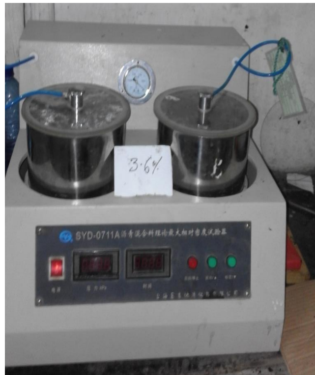
Gmm samples under vacuum suction
