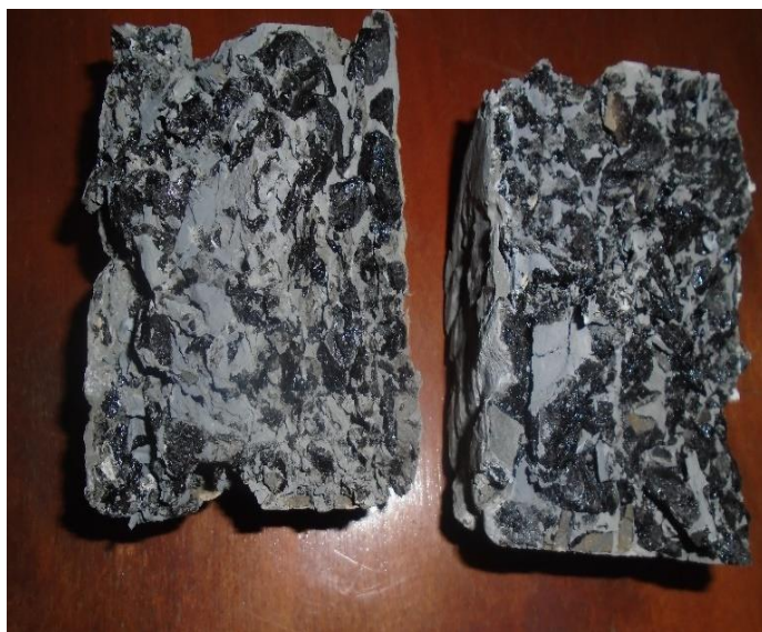
Close-up view of the internal structure of grouted macadam specimen after ITS test
