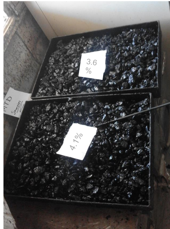
Loose samples for max. theoretical specific gravity (Gmm)
