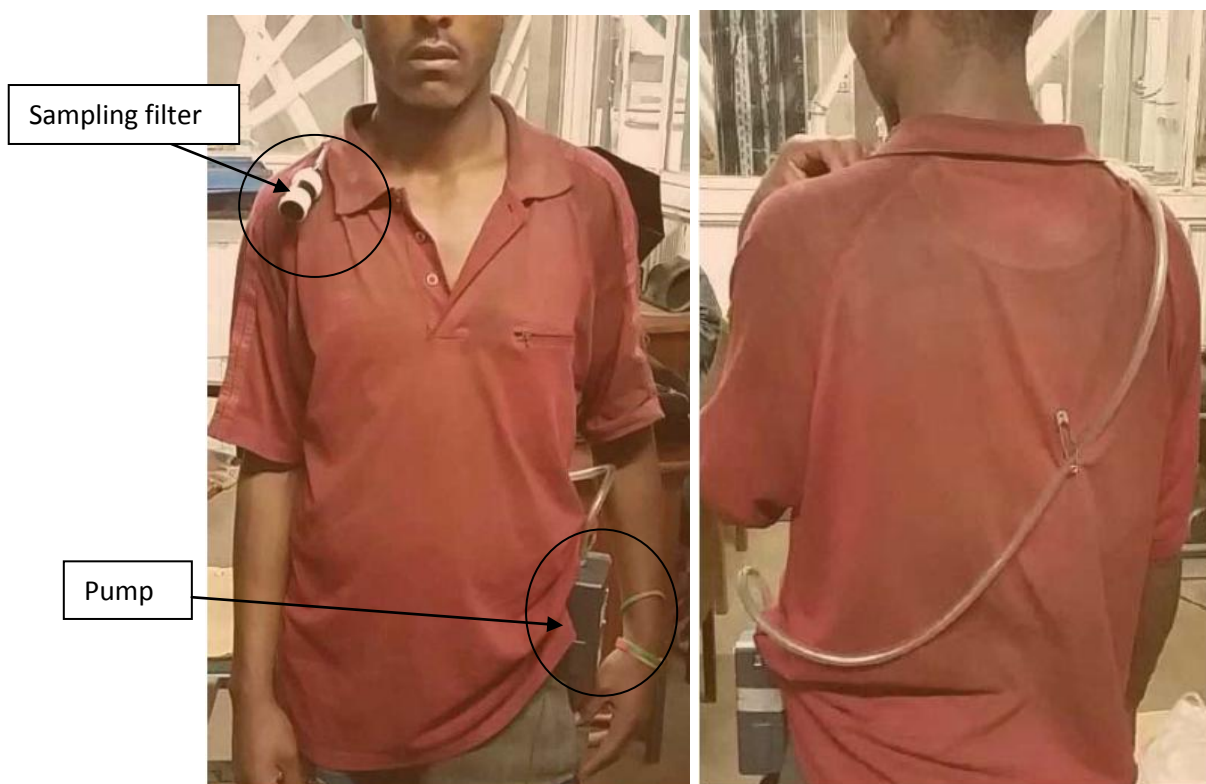
Figure 9: Personal total dust sampling method from breathing zone, right hand person
