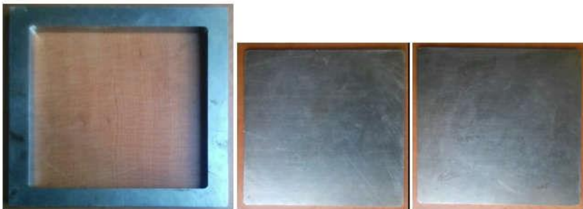
Figure 3-2: Sample preparation mold
