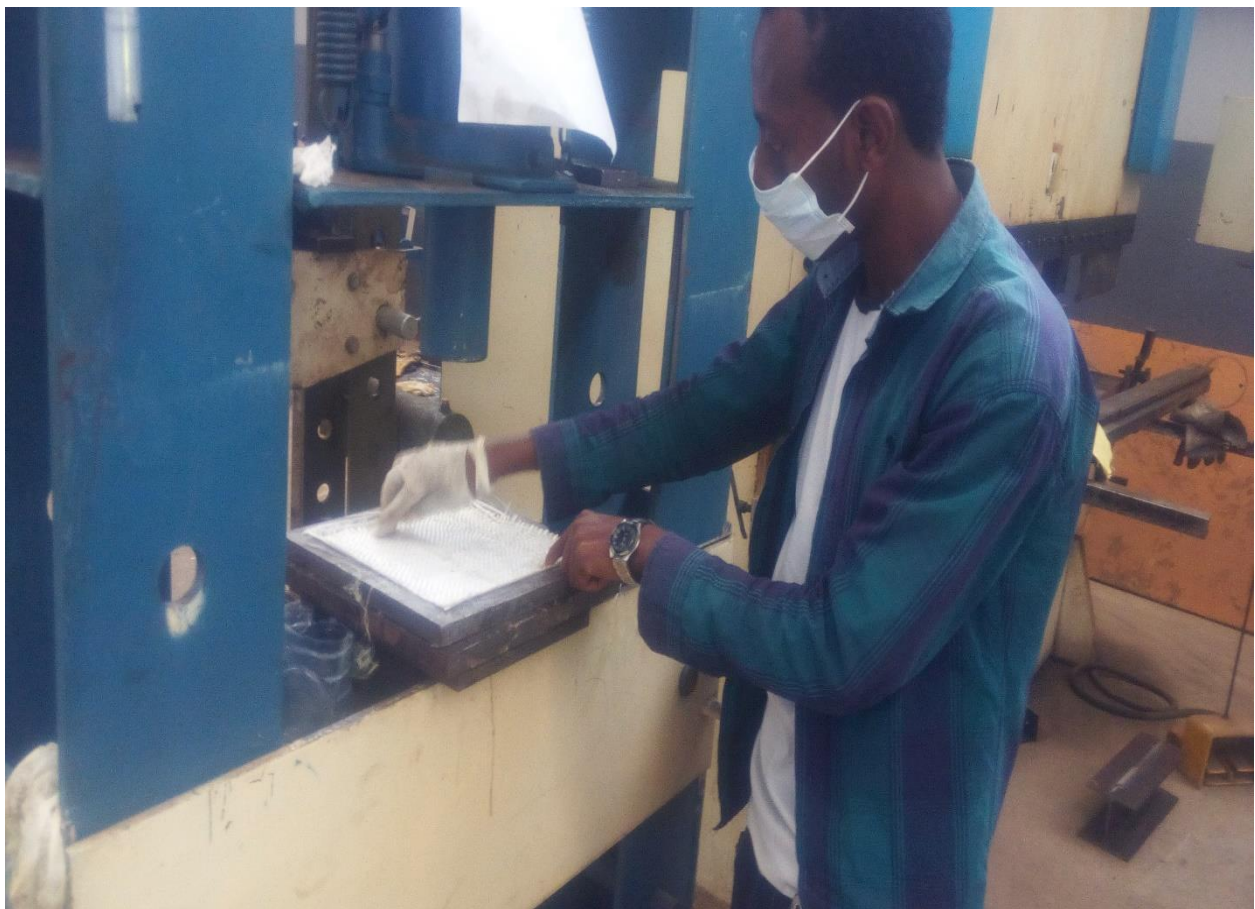
Figure 3-5: Hand layup manufacturing
