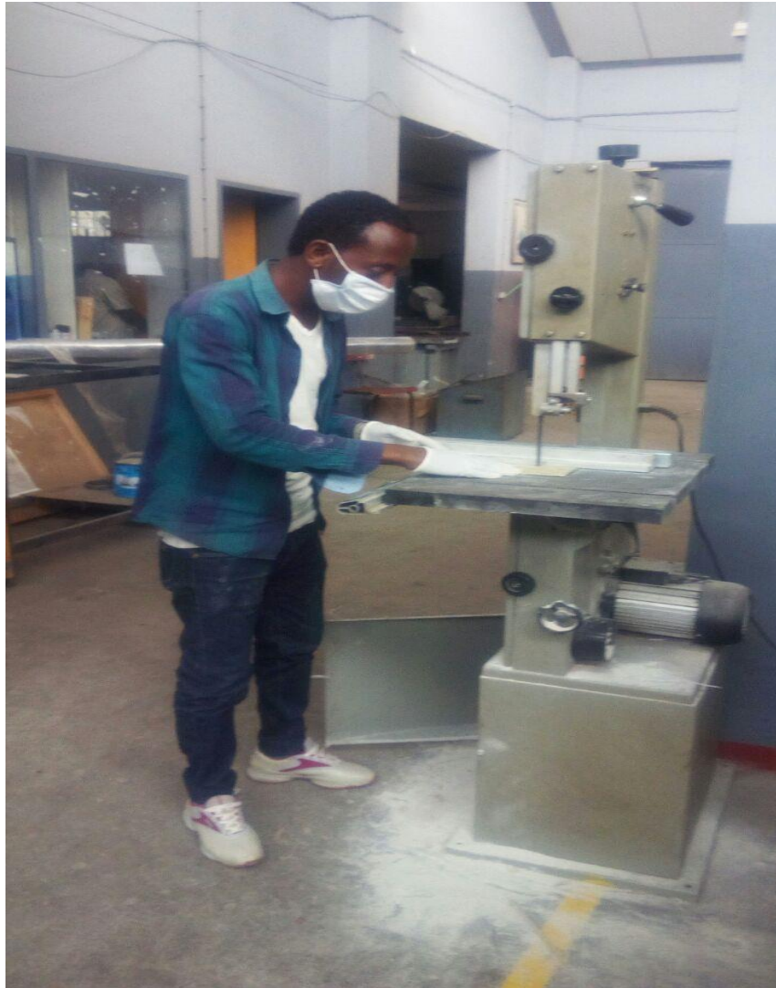
Figure 3-8: Band saw cutting specimens
