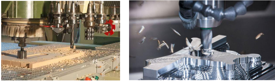
Figure 2.80. CNC Timber Routing of Formwork (Dimar, 2014) – Left and A Machine Subtracting A Metal (Roberson MC, 2022) – Right
