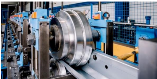
Figure 2.82. Metal Forming - A Cold Forming Operation with Rolls (Voestalpine, 2022) - Left and Glass Slumping – Digital Forming of Glass: (Arzt, 2023) – Right
