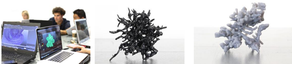
Figure 2.29. Students in the workshop developed algorithmically created geometry studies using physics simulation – left and iterative prints with increasingly complex geometry - right (Formlabs, 2014)
