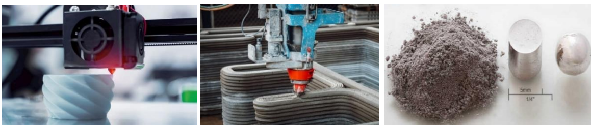
Figure 2.78. Additive manufacturing method (ABB, 2020) - left and Additive concrete construction method (Kauppila, 2023) – Middle and additive metal manufacturing method (Treatstock, 2023) – right
