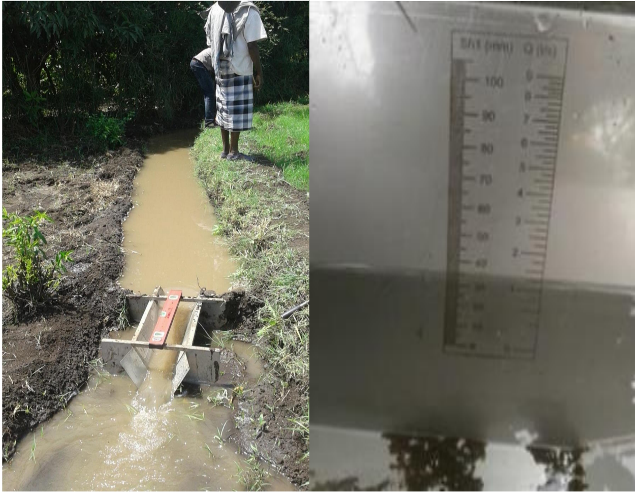
Appendix figure 7. 9: Field discharge measurement by Parshall flume
