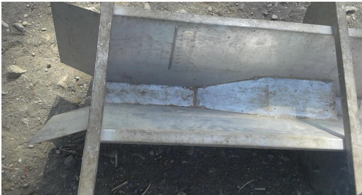
Appendix figure 7. 5: Water flow rate measurement device (Parshall flume)
