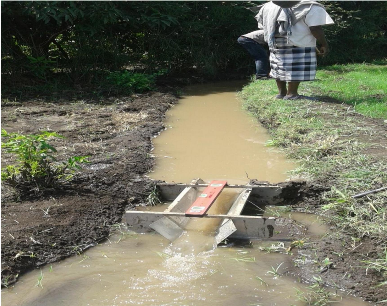
Appendix figure 7. 8: Alignment of Parshall flume
