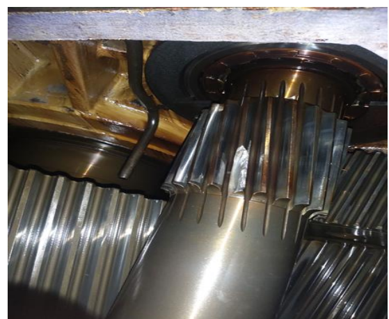
Gear tooth pitting Adama wind Farm II
