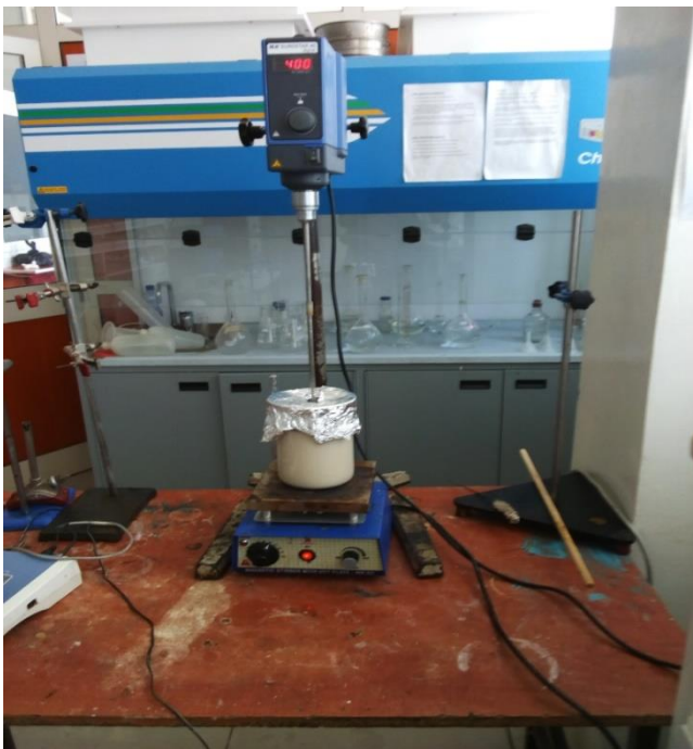
Fig. impregnation of iron and bentonite
