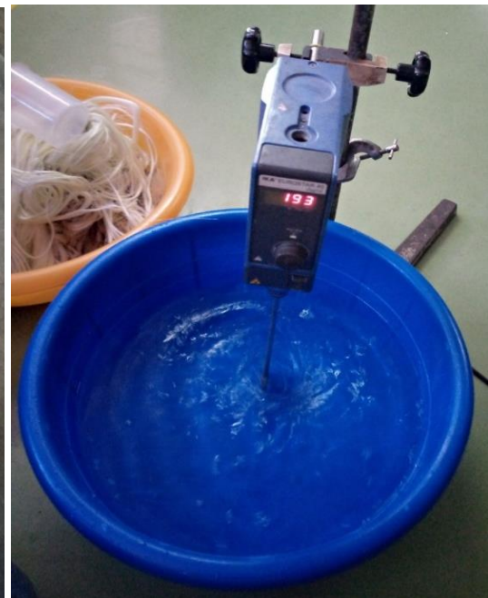
(b) Mixing of NaOH with Water
