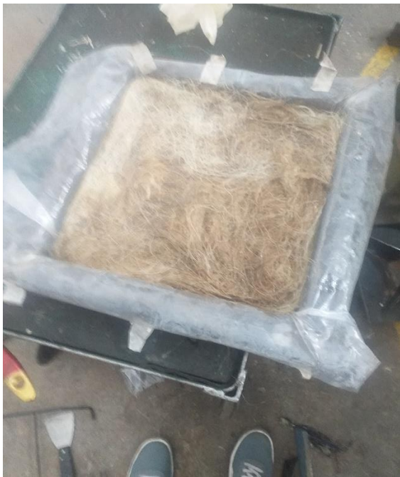
(e) Placing fibers and mixed matrix on mold (f) Applying cover on Mold Base
