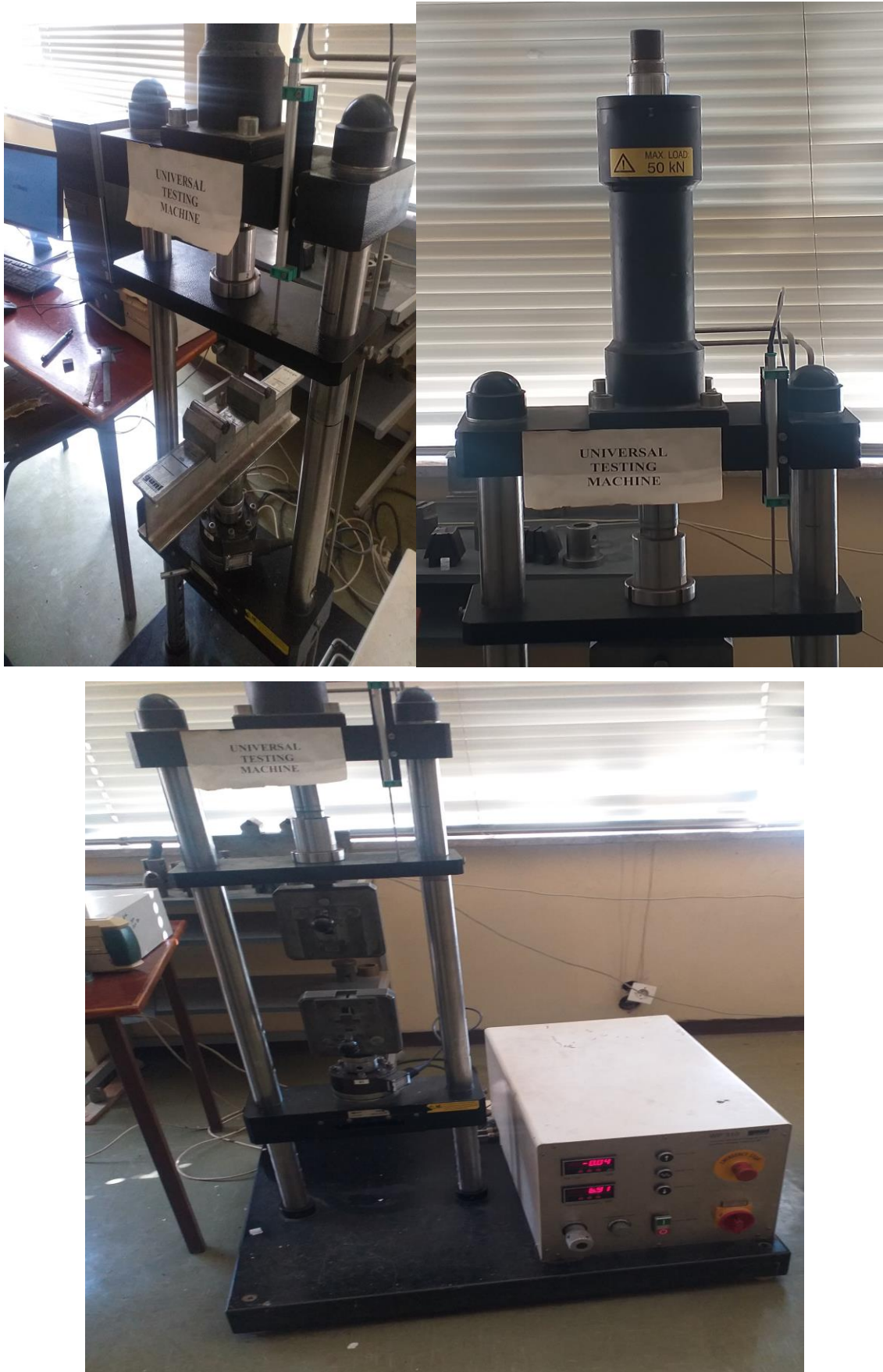
Figure 3. 15 Gunt Hamburg WP 310 Hydraulic material testing machine 50KN
