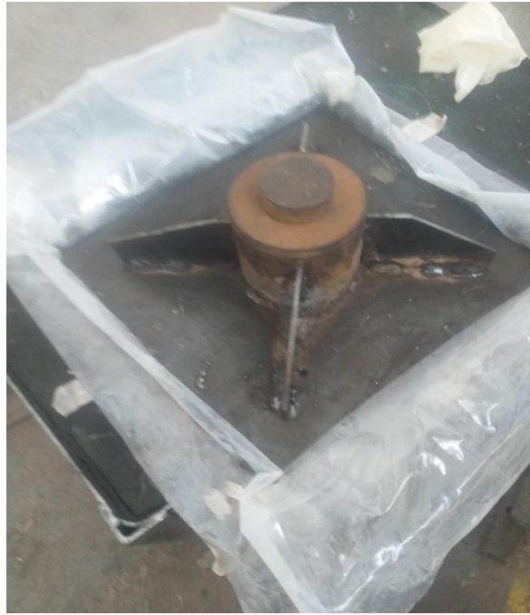
(e) Placing fibers and mixed matrix on mold (f) Applying cover on Mold Base
