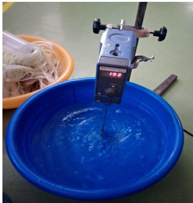
(c) Mixing the NaOH with water using Electric Stirrer
