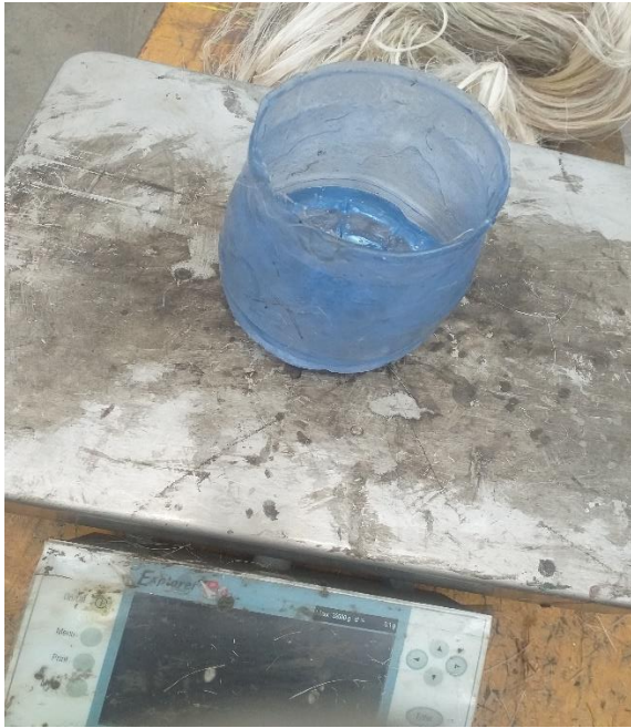
(a) Mixing Epoxy and Hardener
