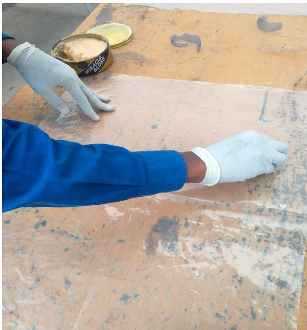
(c) Applying Wax on Plastic Sheet
