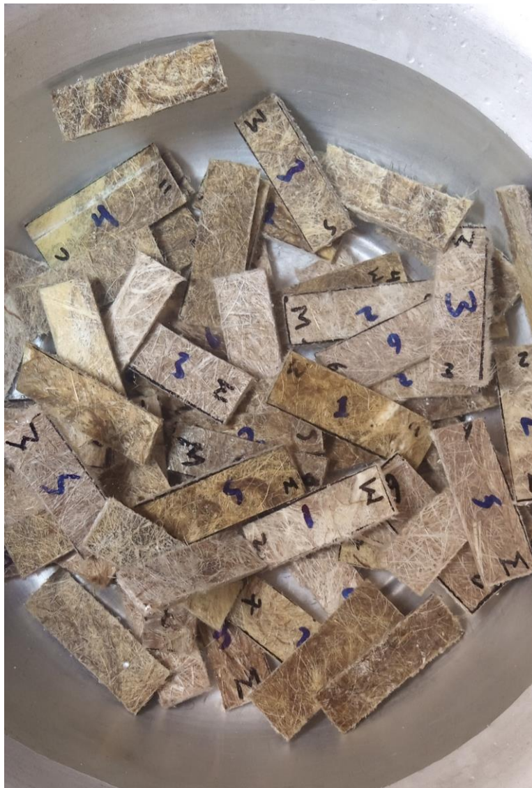
Figure 3. 27 Specimens Socked in Water
