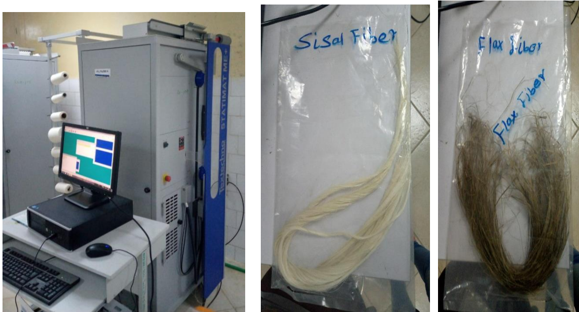
Figure B.1 Flax and Sisal Fiber Ready for Testing of Elongation, Tenacity, Tensile
