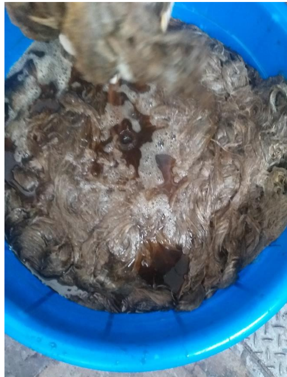
(d) Removal of Flax Fiber from NaOH Solution
