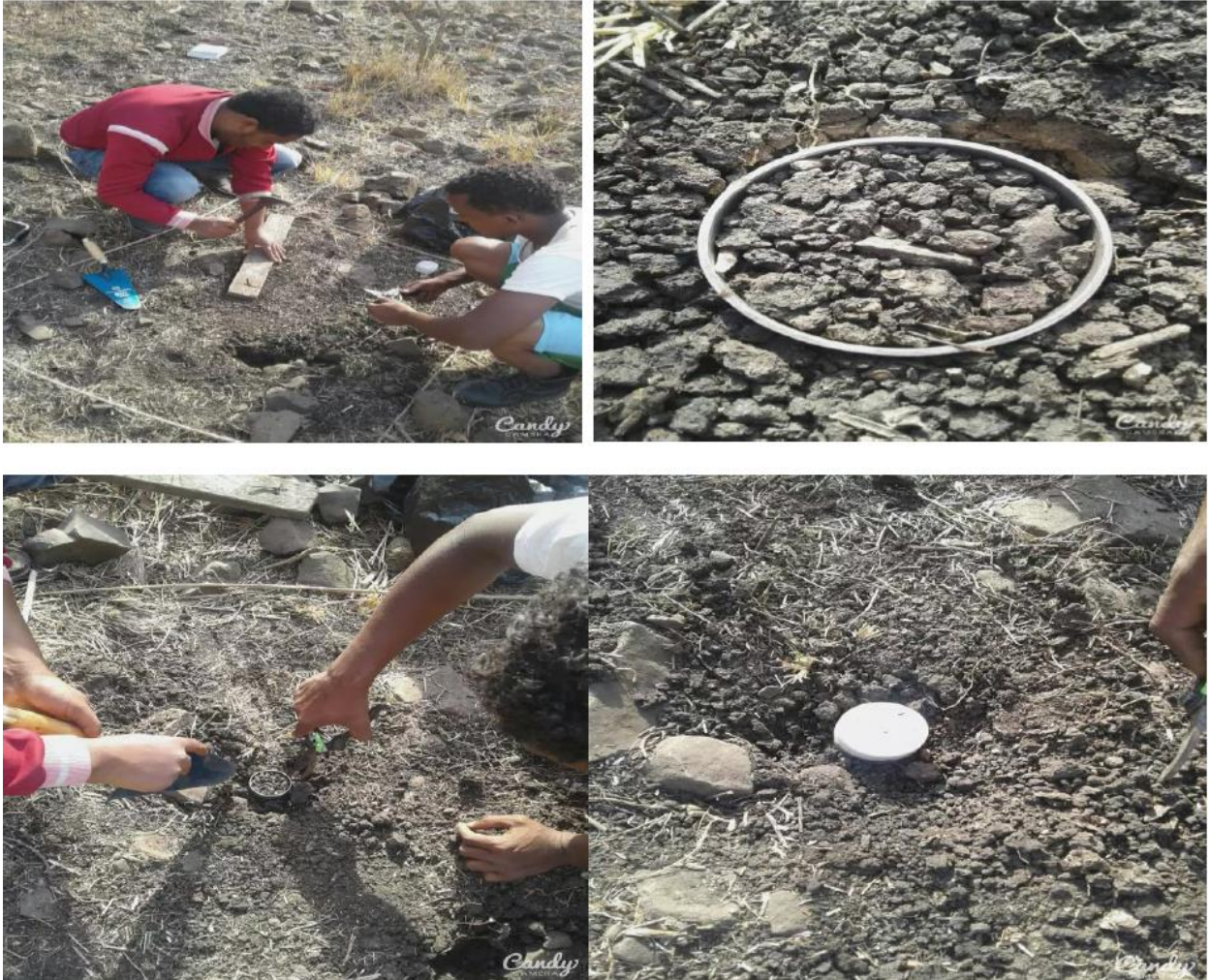
Figure 7 Soil sampling using core sampler for soil bulk density and soil water content measurement.
