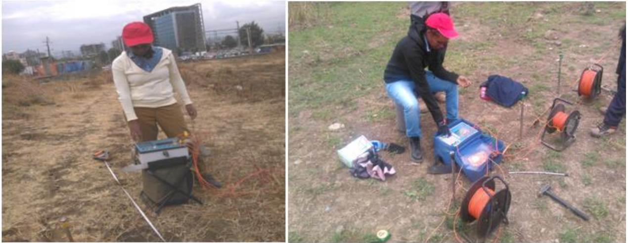
Figure 4.6 field data acquisition of ERT and VES
