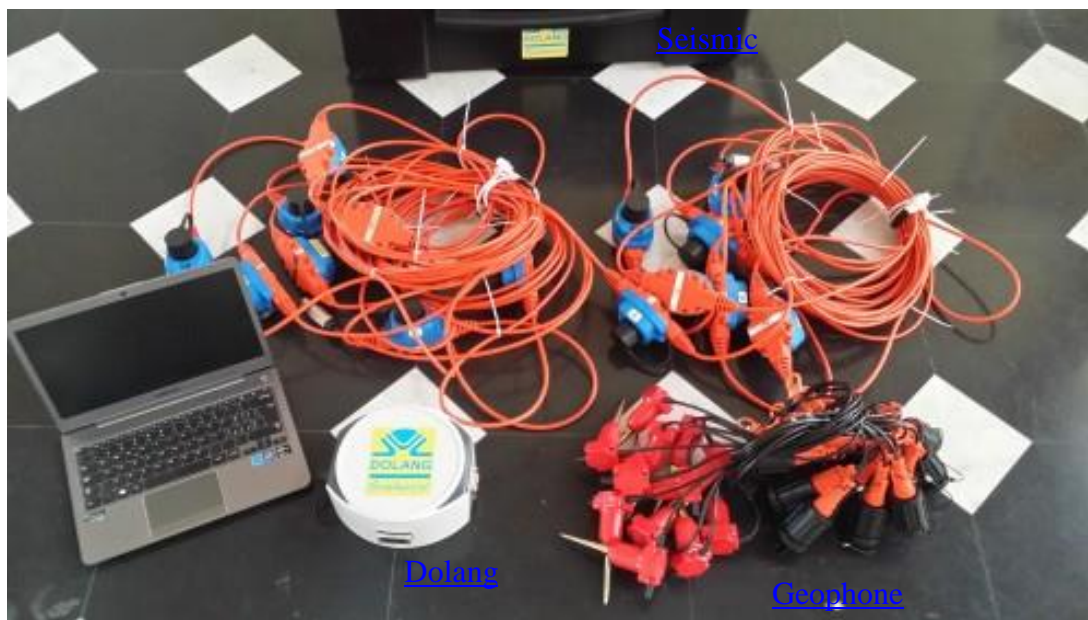
Figure 4.2 Instruments used for collecting seismic refraction data
