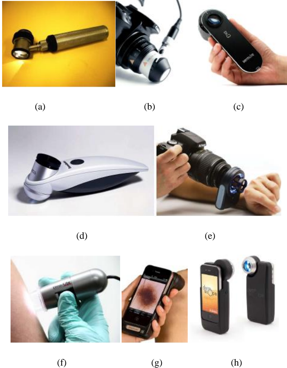
Figure 4.1: Figures (a), (b), (c), (d), and (e) are analog dermoscopies and all except (a) are attachable to digital cameras to function as digital dermoscopes. Figures (f), (g), and (h) are modern digital dermoscopes (Pictures courtesy of Maryam Sadeghi, [28]).
