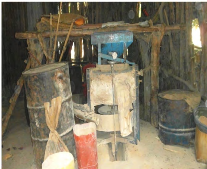
Fig 5.7 diesel flour making milling machine in Deck island
