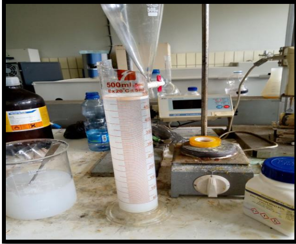
Figure 4: Shows Preparation of DMS solutions for sink-float tests
