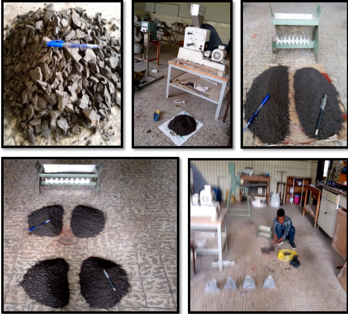
Figure 2: Shows crushing and quartering of coal sample for next laboratory tests and analysis
