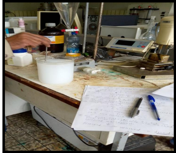
Figure 4: Shows Preparation of DMS solutions for sink-float tests
