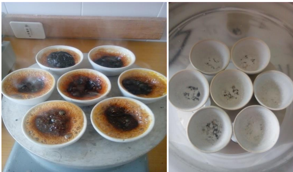
Annex 9: ASH Analysis using muffle furnace.
