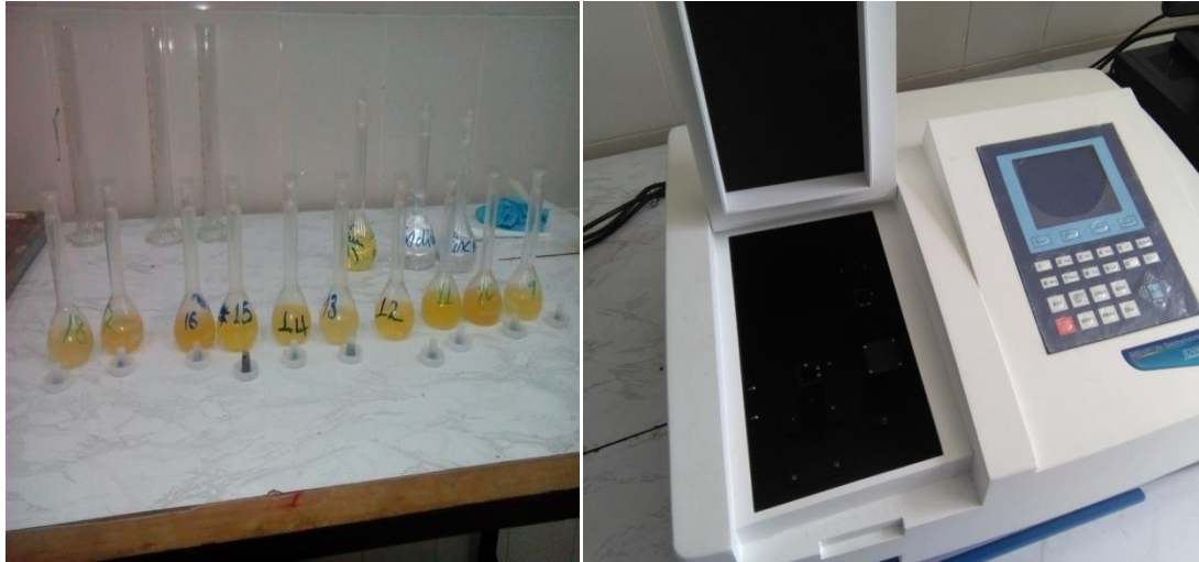
Annex 8: HMF content determination using UV- Spectrophotometer
