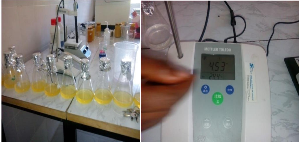
Annex 10: Analyzing free acidity and pH content of the honey samples by using pH meter
